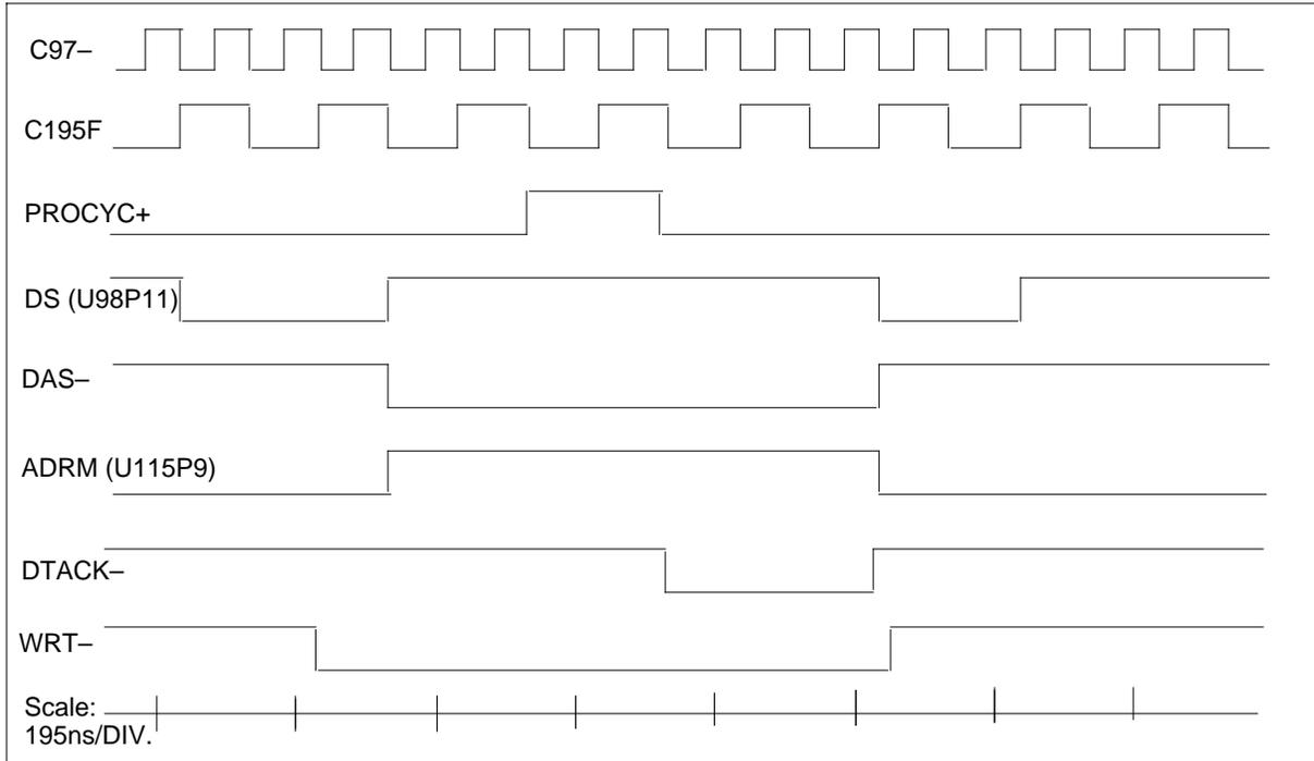
**NT6X69LB A-bus interface timing: FP read cycle**
