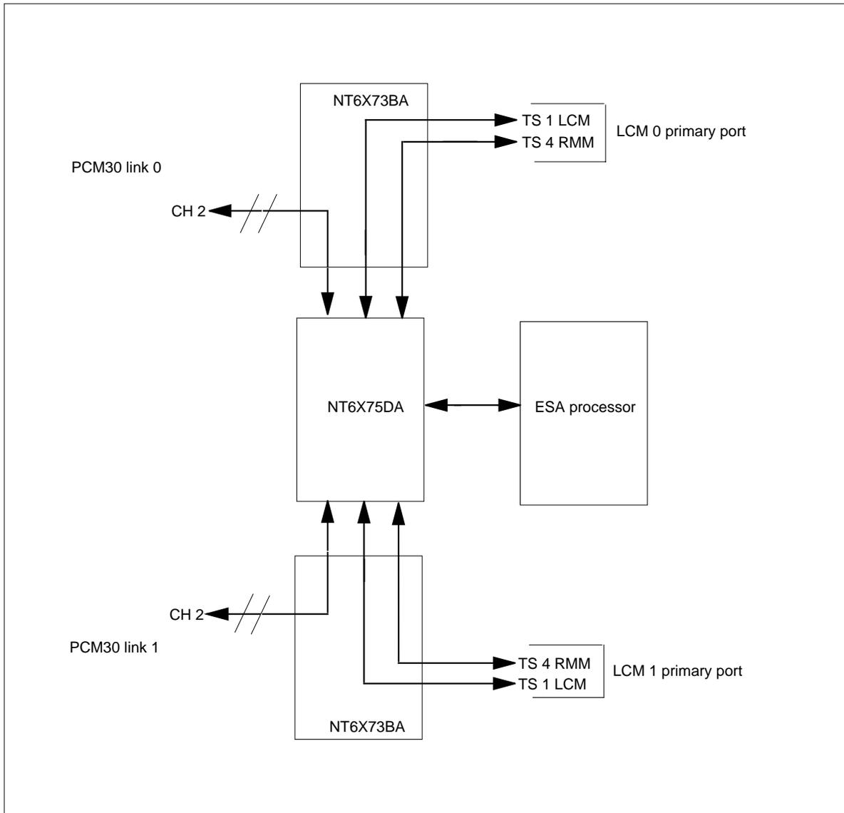
When the LCC is in ESA mode, time slot 1 from each LCM switches to the NT6X75DA from its normal PCM30 path. The ESA processor replaces the LGC as the host and the LCM continues to function as before.
