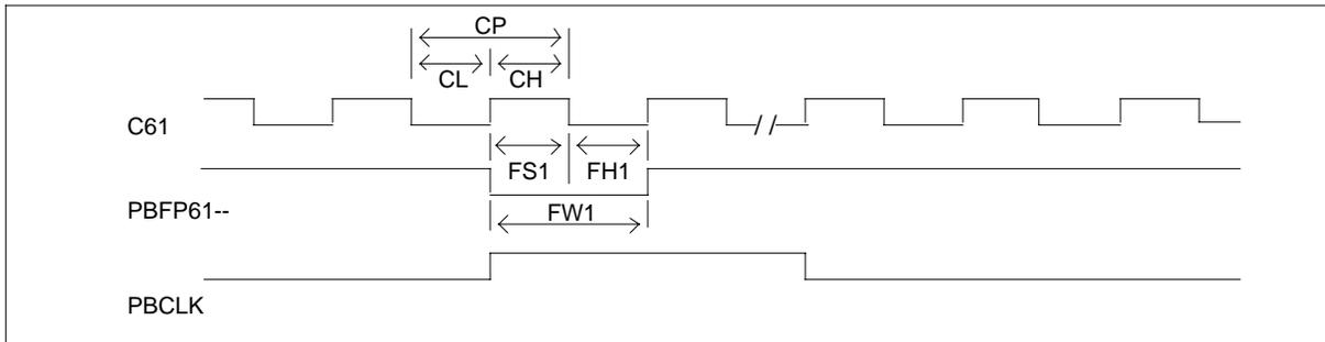
**16.384 MHz clock input timing (Sheet 1 of 2)**
