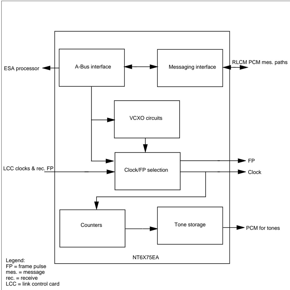
The NT6X75EA circuit card interfaces with the ESA processor in the ESA subsystem. This interface occurs through circuits on the NT6X75EA circuit card which conforms to the A-Bus standard. The ESA processor provides control information for adjusting the voltage controlled crystal oscillator (VCXO) and selection data for selecting the clock source which synchronizes the VCXO, clock and frame pulse signals.
