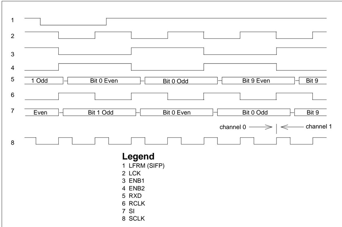
The serial output port channel timing appears in the following figure.
