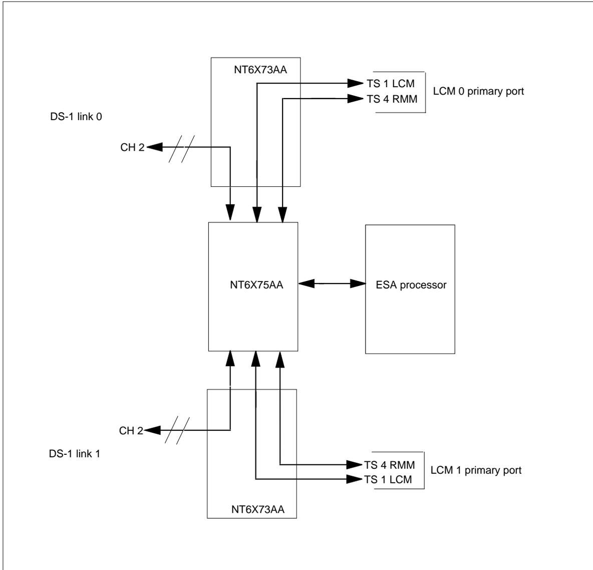
When the LCC is in ESA mode, time slot 1 from each LCM switches to the NT6X75AA from its normal DS-1 path. The ESA processor replaces the LGC as the host and the LCM continues to function as before.
