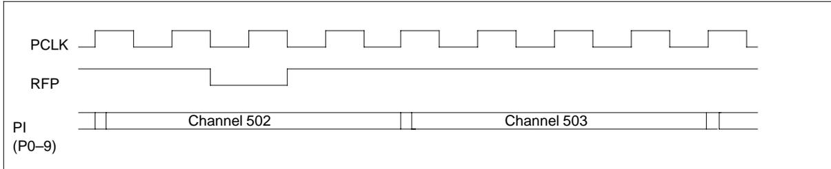
**Parallel output link channel timing**
