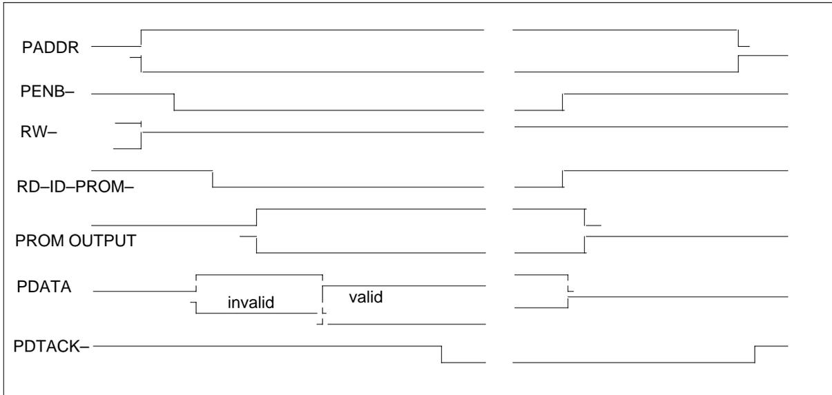
The maintenance register read timing appears in the following figure.
