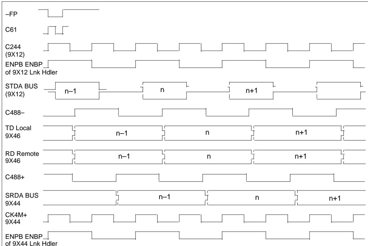
The link data transfer of NT9X4402 to NT9X12 timing appears in the following figure.
