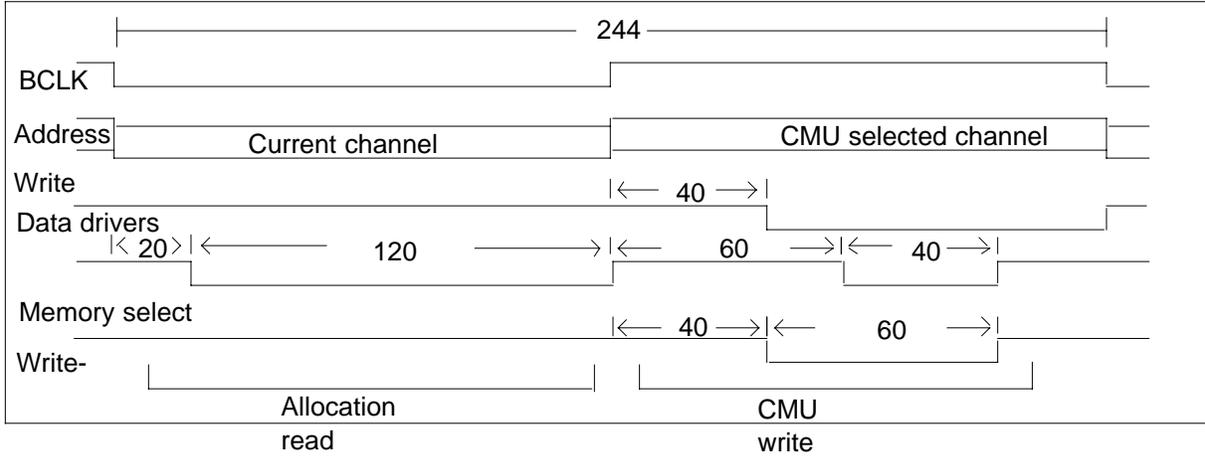
The CNM RAM cycle with CMU read timing appears in the following figure.
