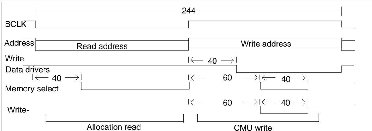
The CNM RAM cycle with CMU write timing appears in the following figure.
