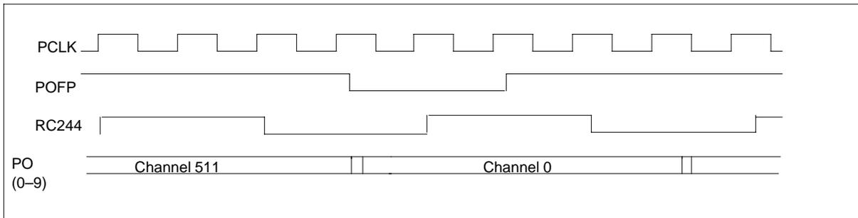
**Serial input link channel timing**
