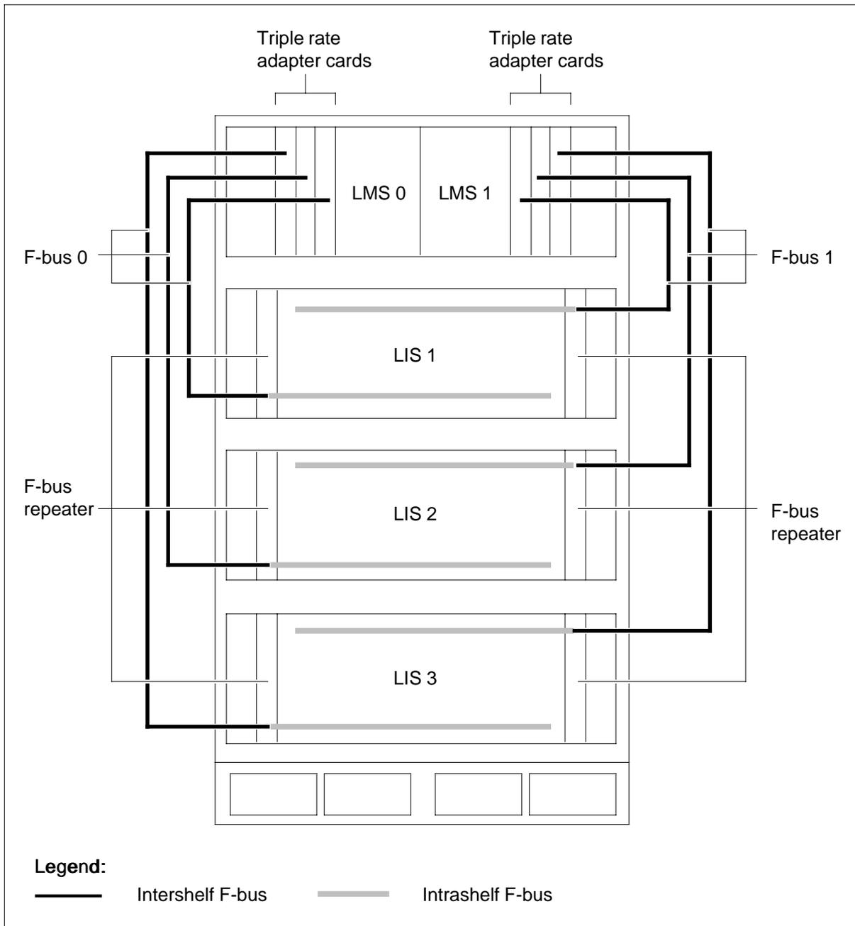
Each LIS can house up to 4 DLIUs, which means a total of 12 DLIUs in an ELPP cabinet. The DLIU terminates and processes messages that enter and leave the ELPP through DS-1 (1.544 Mbit/s) signaling data links.
