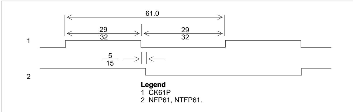
The DS30 clock and frame pulse timing appears in the following figure.
