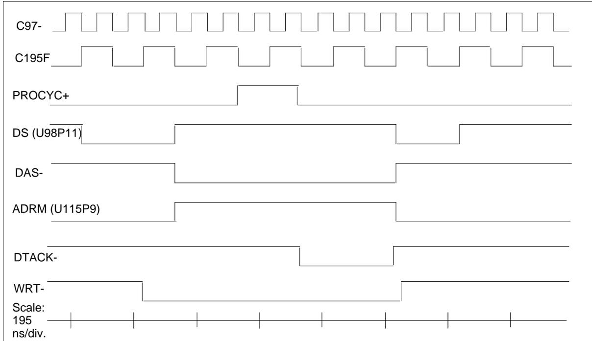
**NT6X69MA A-bus interface timing: SP read cycle**
