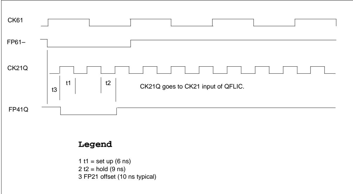
**NT9X62AA Out-of-band serial format to the backplane timing**
