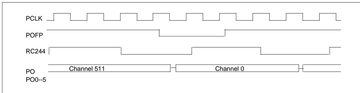
**NT9X69AA serial input port channel timing**
