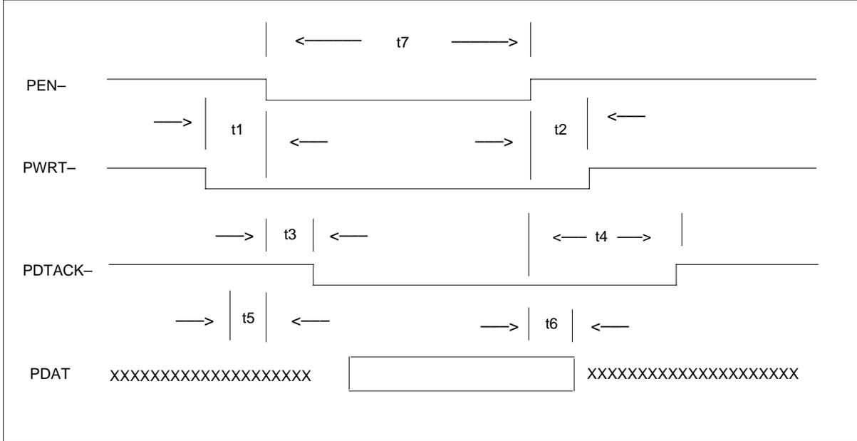
**P-bus interface timing (write cycle)**
