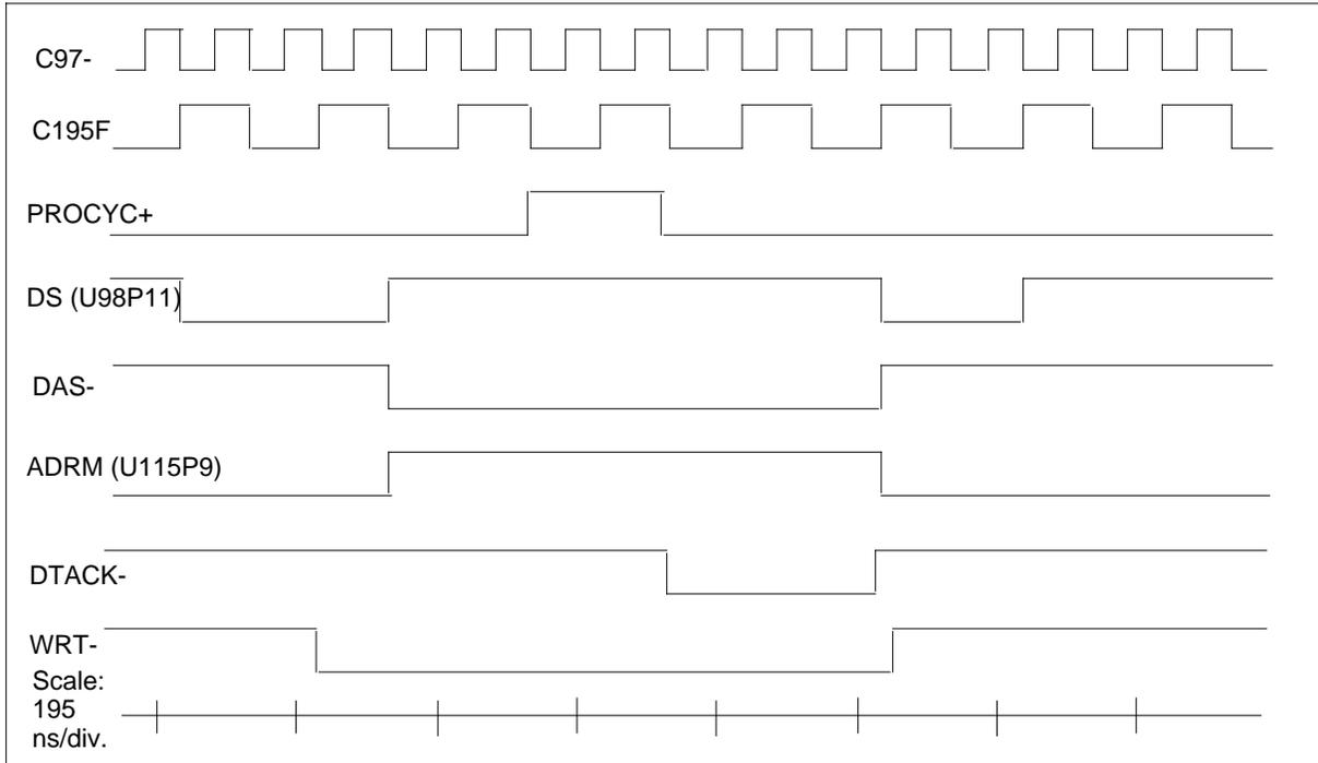
**NT6X69LA A-bus interface timing: FP read cycle**
