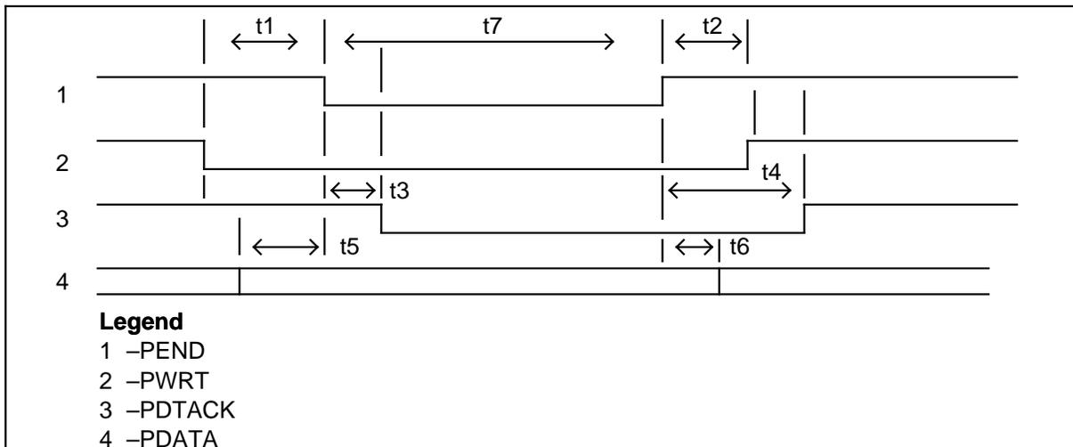
**NT9X25AA processor READ cycle timing**
