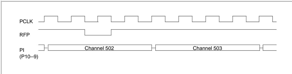
**NT9X69AA parallel output port channel timing**
