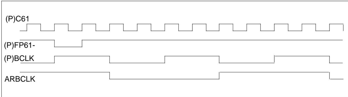
The RAM control signal timing appears in the following figure.
