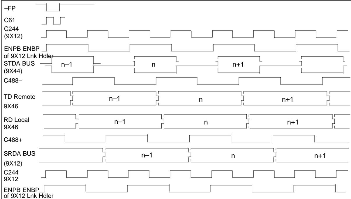
The local data loop of NT9X12 to to NT9X12 timing appears in the following figure.
