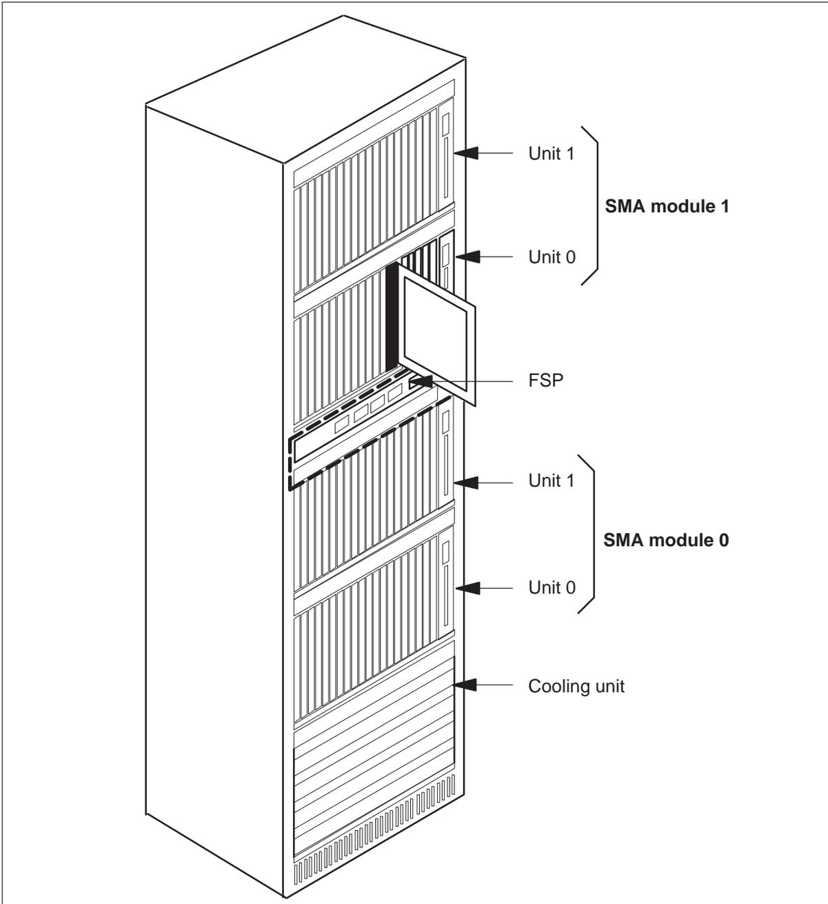
Two to ten DS-1 interface cards are distributed across both shelves of an SMA module. The interface cards provide a maximum 20 DS-1 ports that
