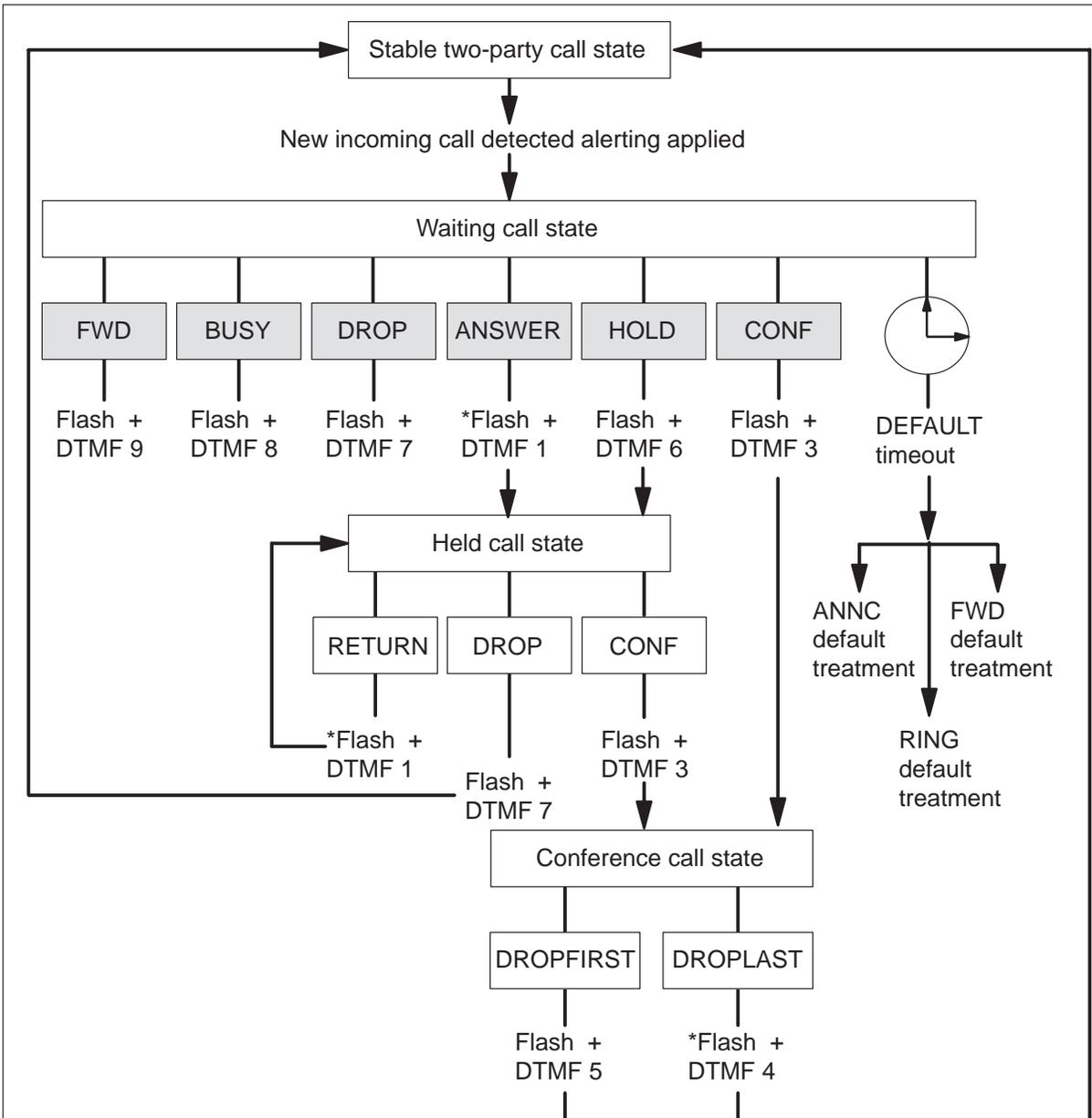
**Note 1:** An asterisk indicates the user can perform a flash to accomplish the same function as the transmission the DTMF code for that digit.
