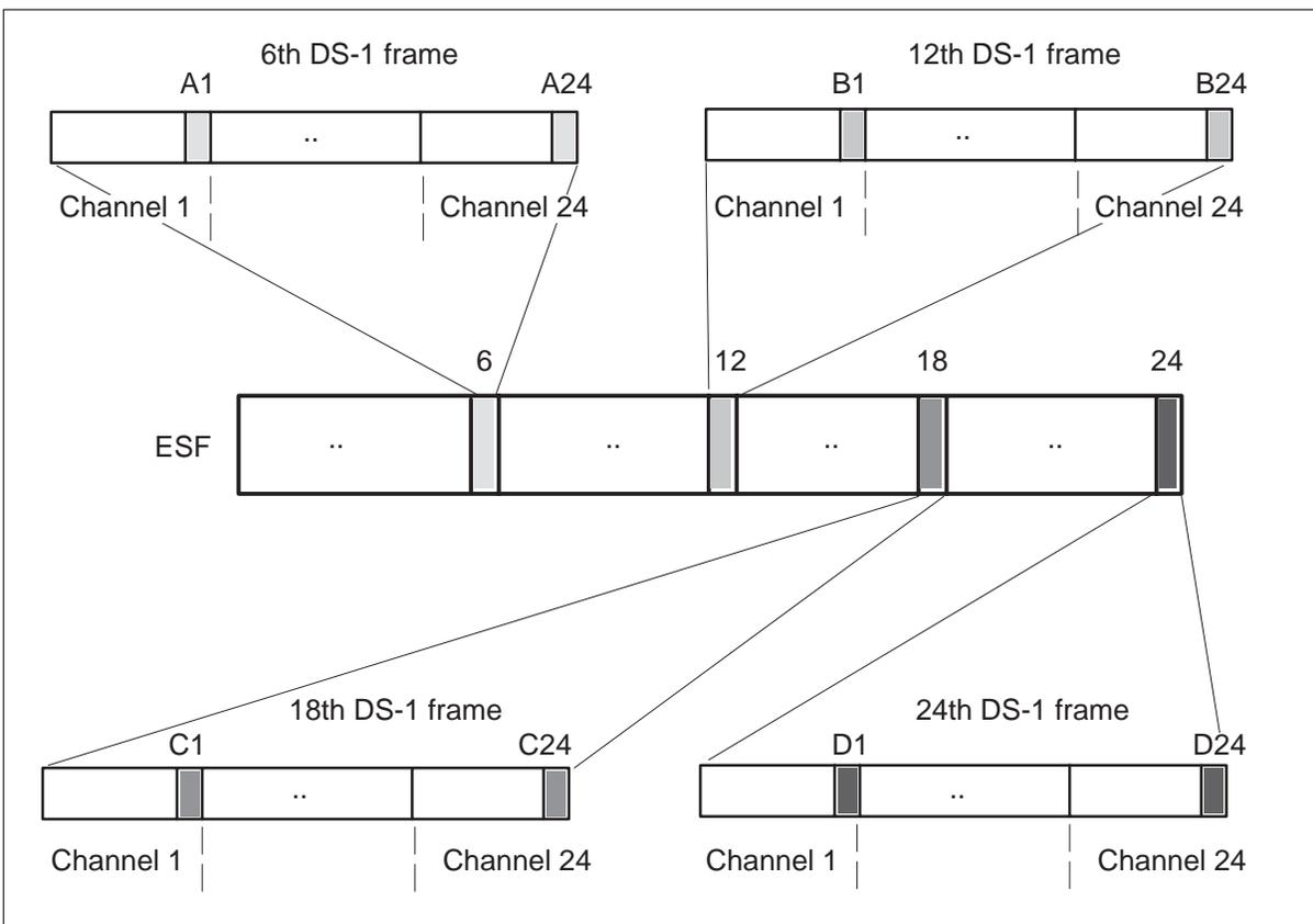
The ABCD bits facilitate the exchange of call supervisory information between the IDT and the RDT. The IDT uses TMC to set up a clear time slot connection at the RDT.
