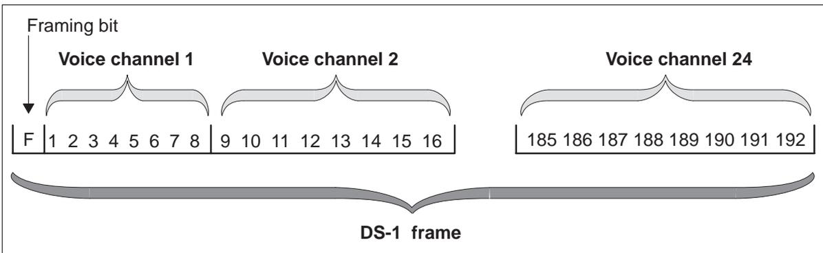
The framing bit identifies the location of the first time slot in the frame. The RDT or SMA can receive a framing bit. When this event occurs, the system notifies the RDT or SMA if the following 8 bits contain information from time slot one. Frame alignment in the extended superframe alignment requires the framing bit.
