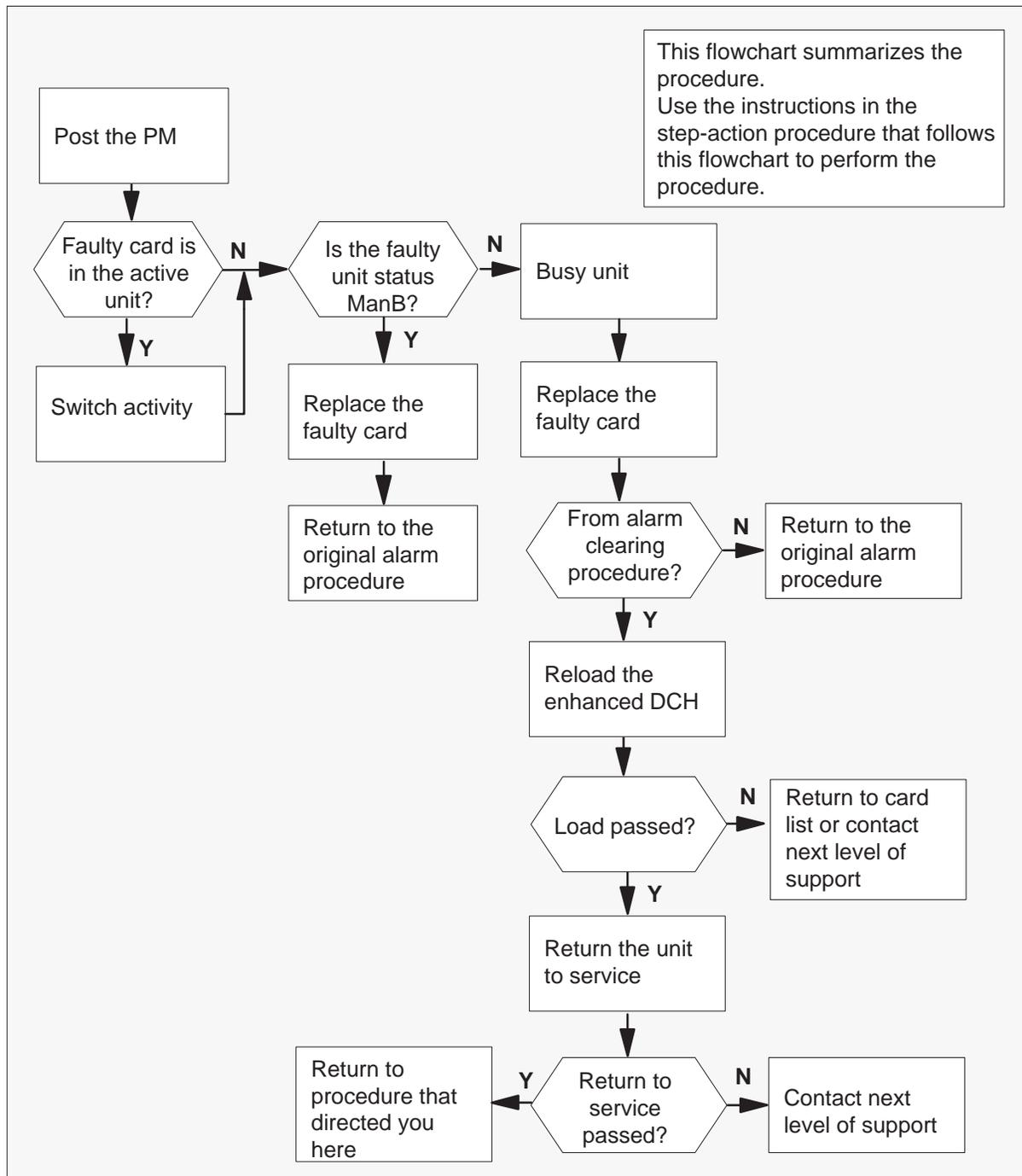
**NTBX02****SMA** (continued)**Replacing an NTBX02 card in an SMA****At the equipment frame**
