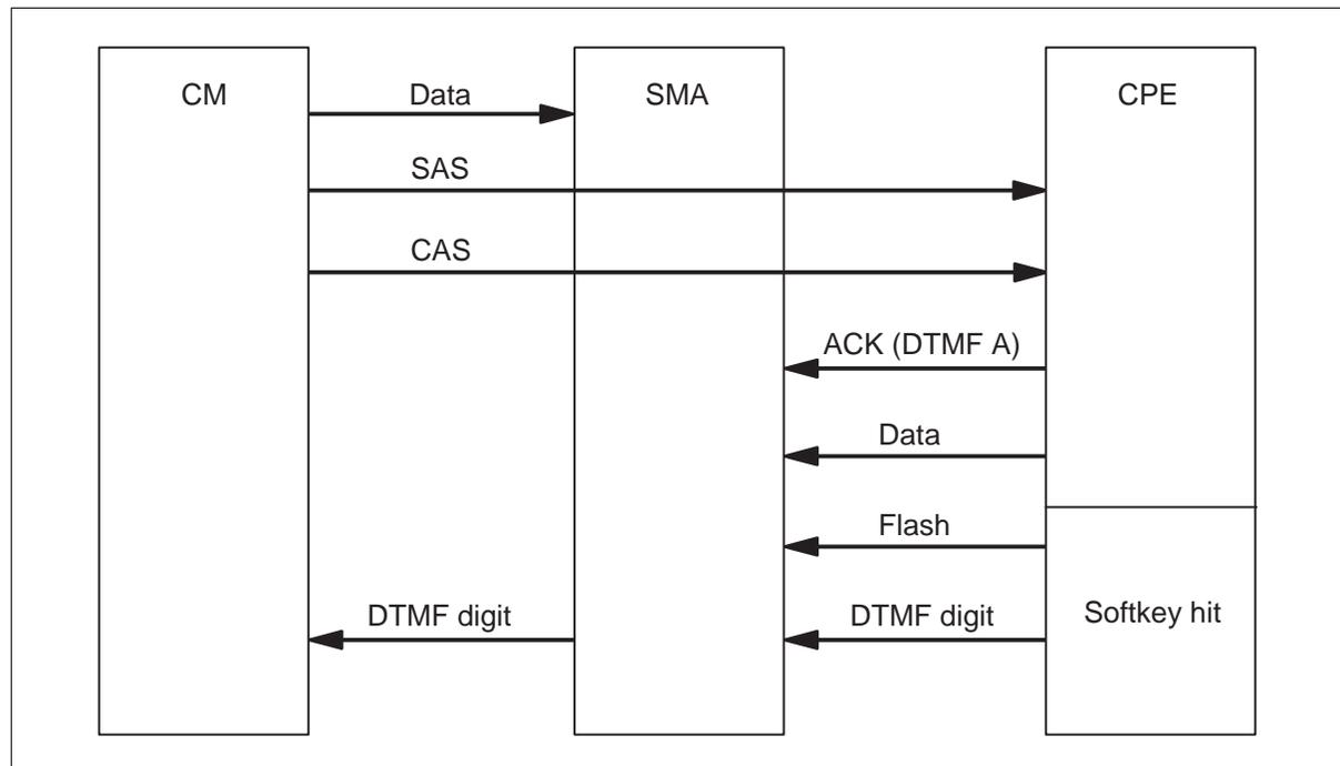
If the CPE is a SCWID CPE, the CPE sends a DTMF D ACK signal in response to the CAS. When the system sends alerting tones, the subscriber can control disposition of the incoming call. To respond, the subscriber can use the softkeys if the CPE is ADSI. The subscriber can use hard-coded keys if the CPE is a SCWID, or a 2500 set. If the CPE does not respond with an acknowledgment tone, the system treats the CPE as a 2500 set.
