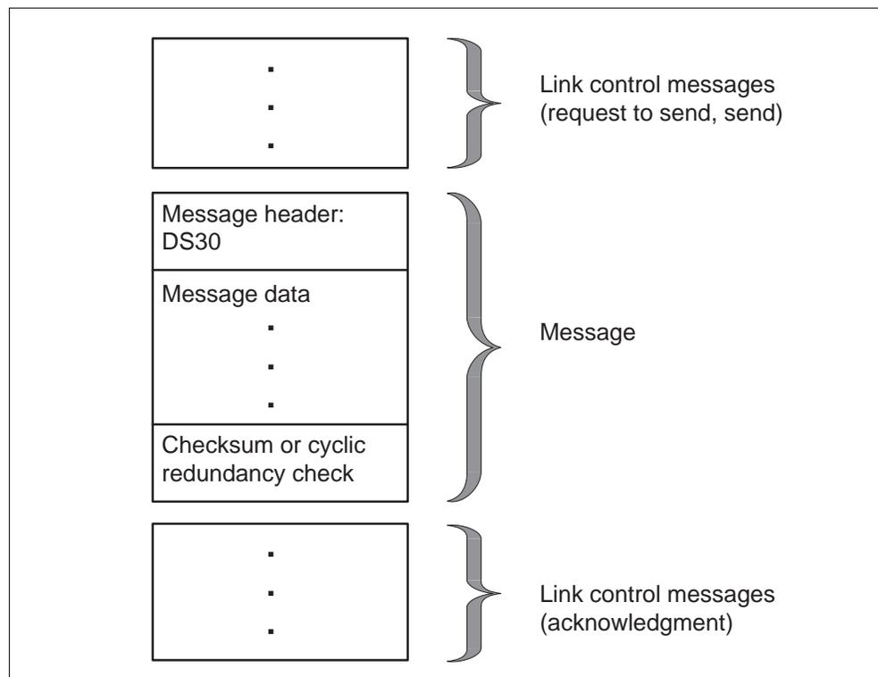
Message time-out, message checksum or CRC calculation perform message error detection. In the event of protocol, checksum, or CRC failure on an outgoing message, the sending node attempts the send sequence again.
