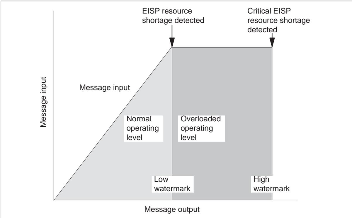
When the system reaches the *low watermark* for resource congestion, the EISP enters the overloaded operating level. The system places logical links on the EOC are placed in the receiver-not-ready (RNR) state. The exception is the logical link used for protection switch control. The RNR state reduces the number of incoming messages.
