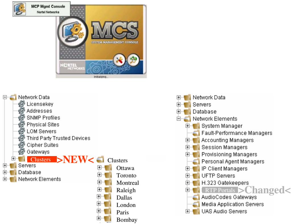
Figure 12 System Management Console: Affected Data Structures
