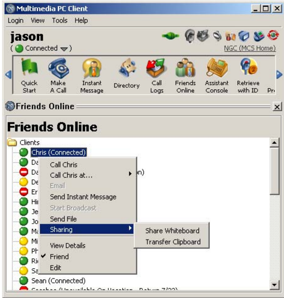
Figure 32 Right-Click Menu of the Friends Panel without the Send Web Page Item
