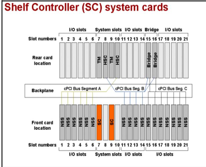
**Note:** In SAM21 SC figure, the Non-system slot cards (NSS) reside in front slots 1-6 and 11-21. Any of the following applications: Call Agent, MC and USP-Compact can also be run on the NSS cards. Refer to the "CS 2000 Compact" hardware section for more information.
