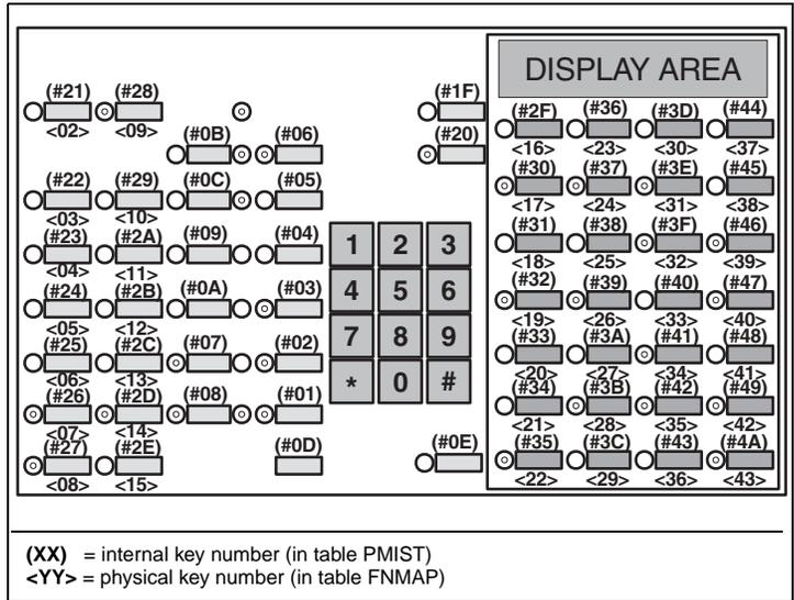
The following figure shows the TOPS MPX IWS keyboard.
