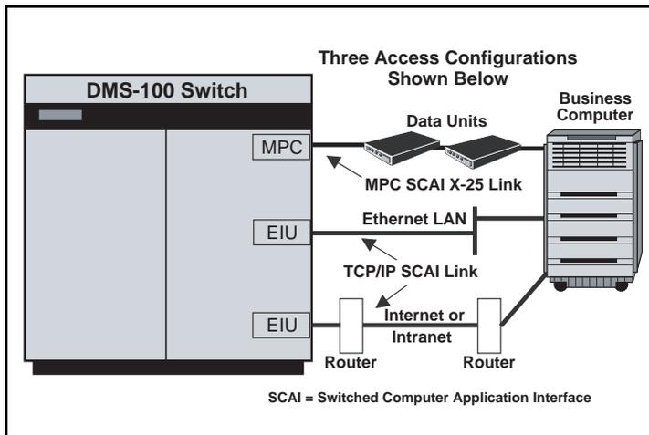
**Note 1:** MPC = NT1X89 Multi-Protocol Controller Card located on the IOC shelf
