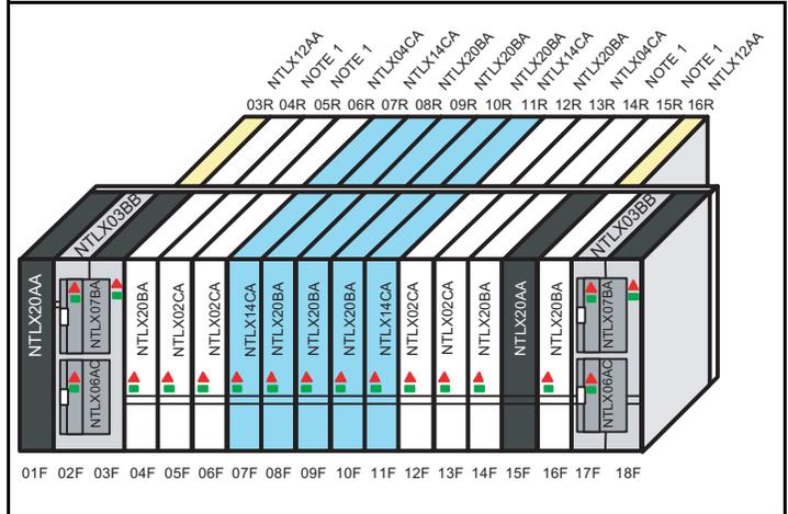
**Note:** Rear slots 4R, 5R, 14R, 15R contain NTLX03AB I/O processors which are populated with NTLX08AB (RTIF) and NTL05AB (CMIC) circuit packs.
