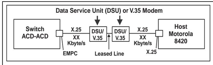
Link requirements when switch and host are co-located less than 100 ca. ft. If the switch and the Motorola 8420 are not co-located, one of the following two options is required:
