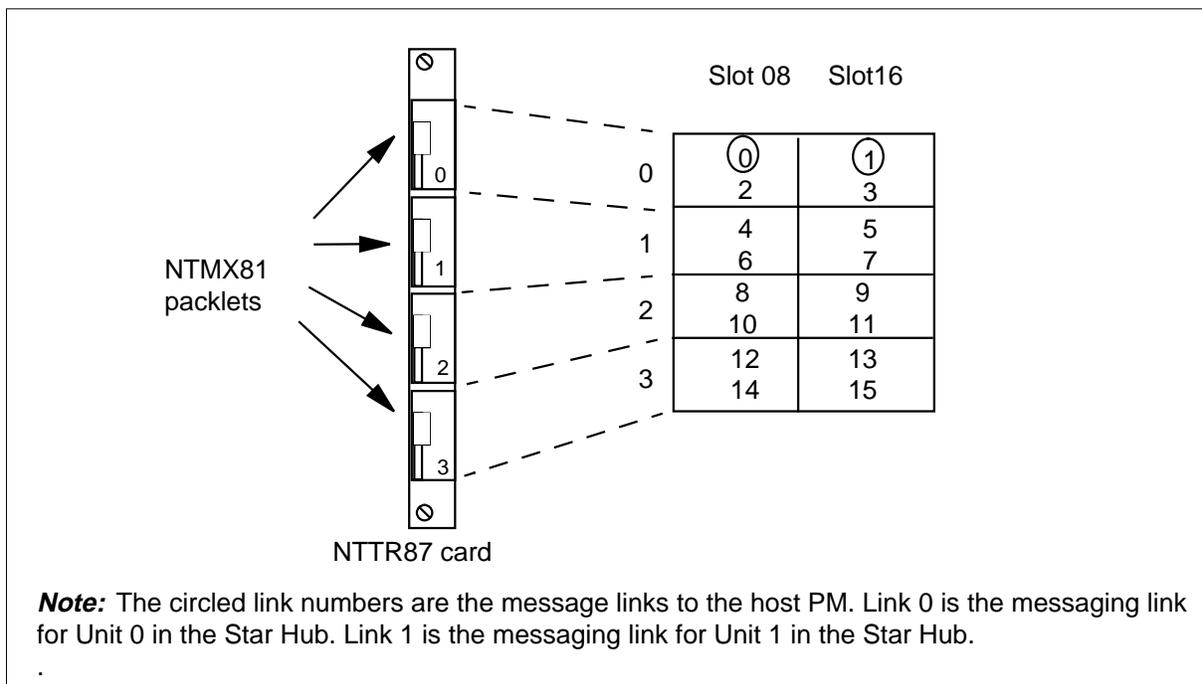
The following figure shows the NTTR87AA quad frame carrier with NTMX81AA packets.
