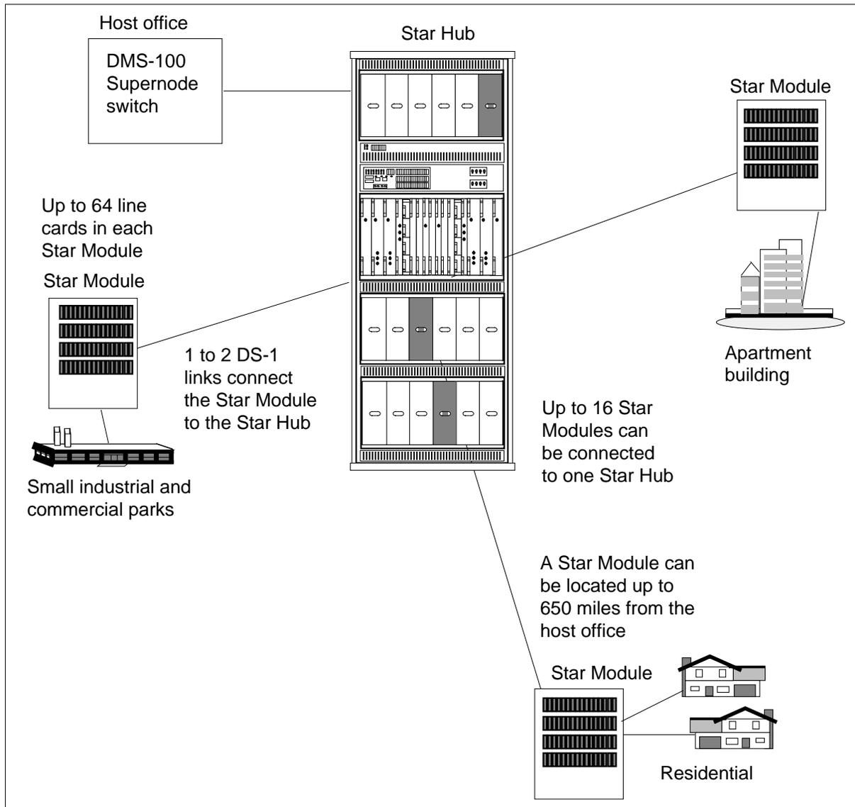
The following paragraphs describe the characteristics and capabilities of each of the Star Module components.
