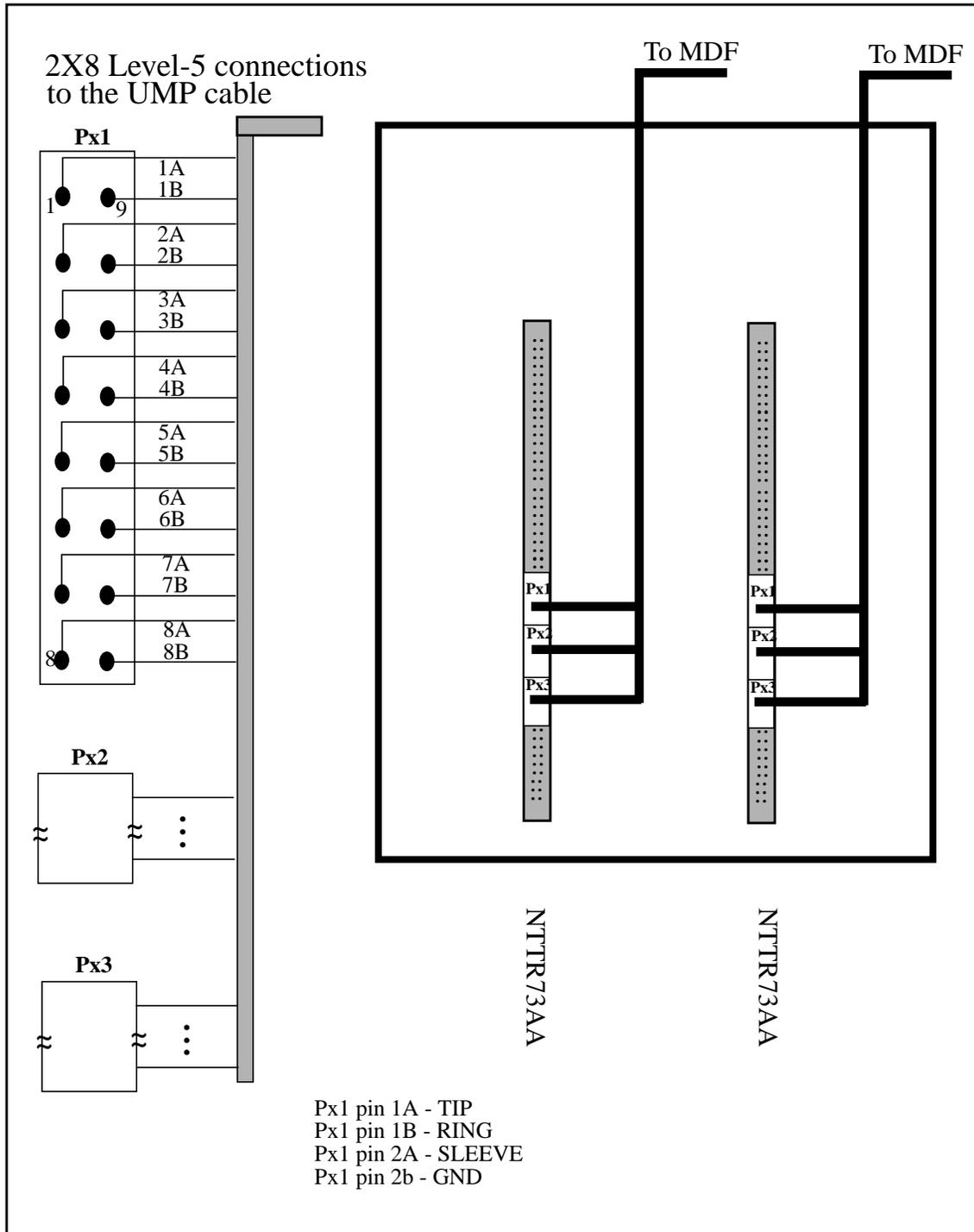
**Note:** There are two UMP to MDF cables in the Star Remote HUB configuration. The UMP cables run to slots 11 and 13 in the controller shelf.
