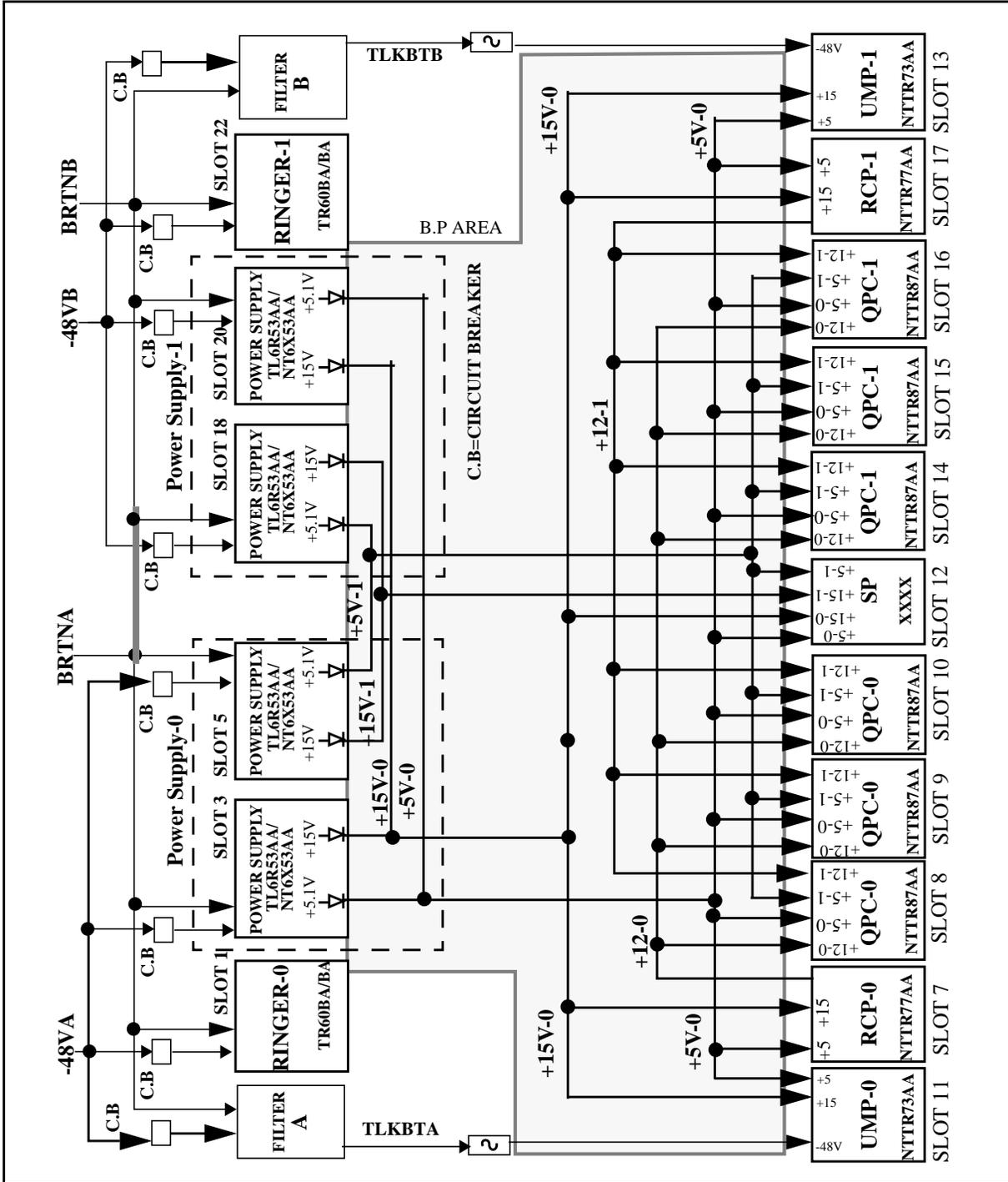
configuration provides a redundancy of power from both power feed sources to each unit of the Star Hub. There is also some redundancy. When the talk battery returns, a single fault may not cause an outage.
