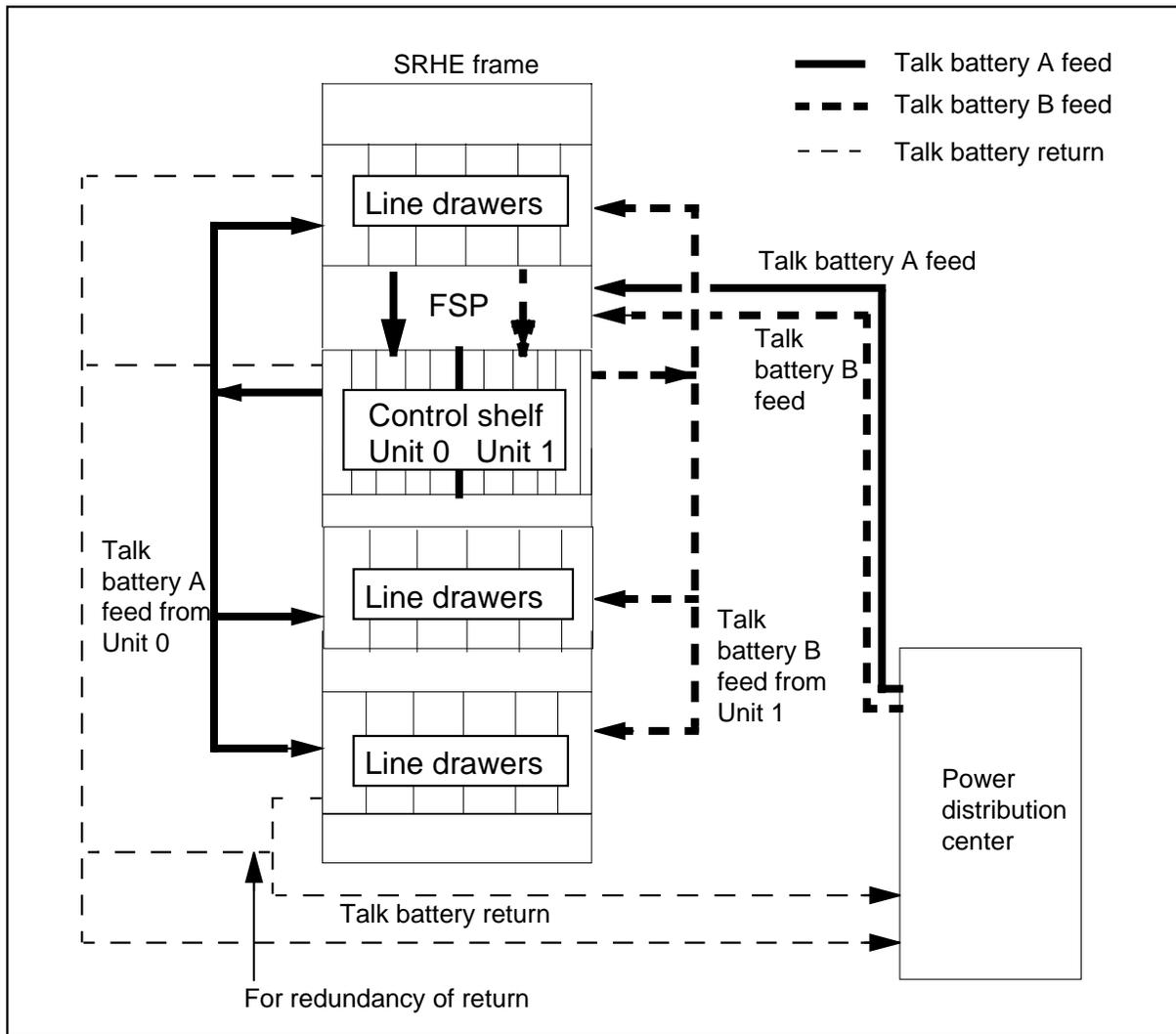
The following figure shows how talk battery distributes within the Star Hub control shelf.
