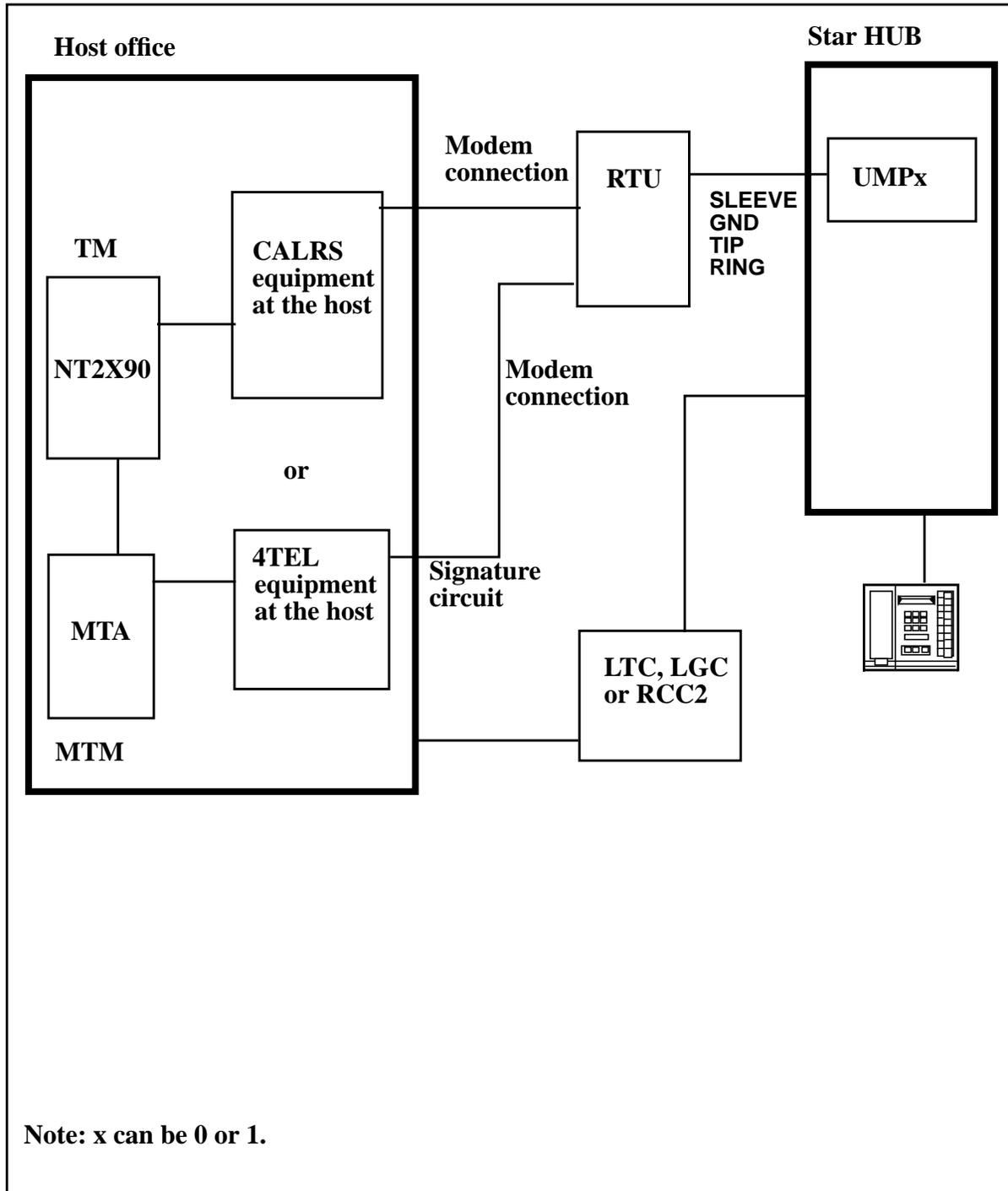
Figure 7-3 Star HUB Line testing configuration with DMS-1U
