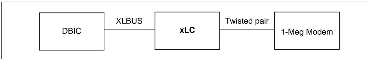
The NTEX17DA supports a transmission rate of 1280 kbit/s downstream and 320 kbit/s upstream. Up to 31 xLC cards can be provided in a line drawer.
