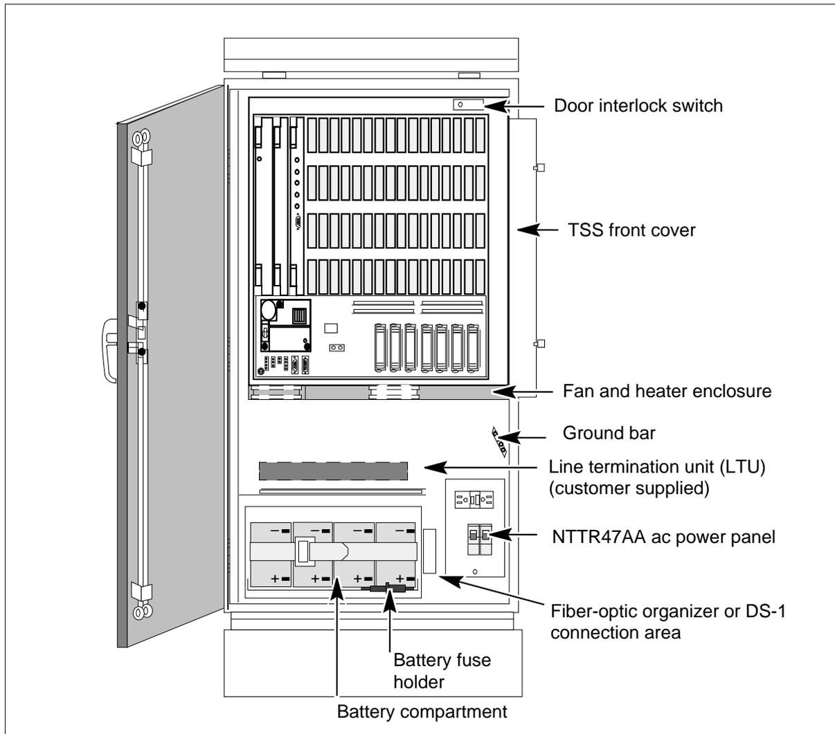
**Batteries** There is one string of four lead/acid sealed batteries. The Star Module in the SRMO cabinet uses Yuasa batteries, type NP18-12BFR, with a nominal capacity of 12 V, 17Ah.
