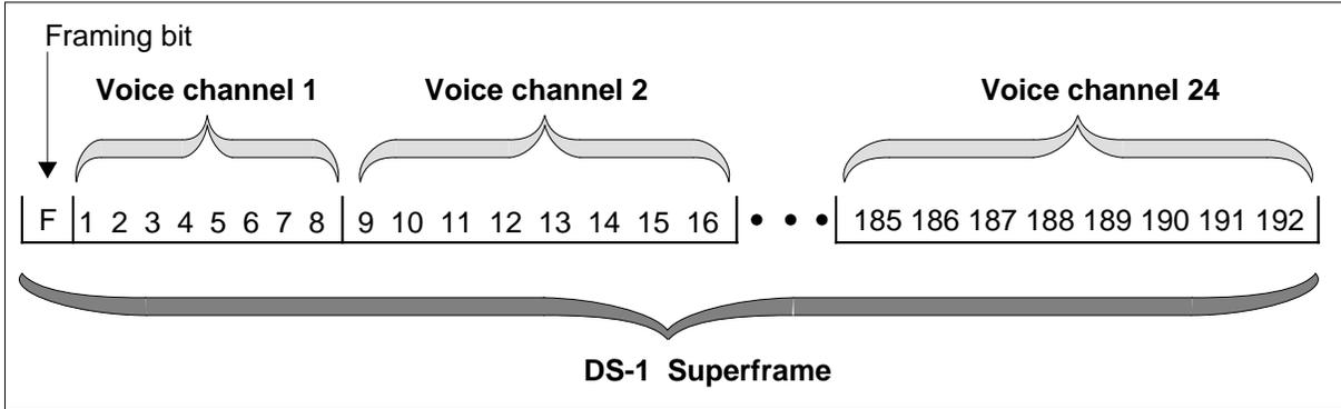
The framing bit identifies the location of the first time slot in the frame. When the Star Hub receives a framing bit, the Star Hub is told the eight bits that follow contain information from time slot one. The framing bit provides frame alignment within the superframe and extended superframe alignment configurations.
