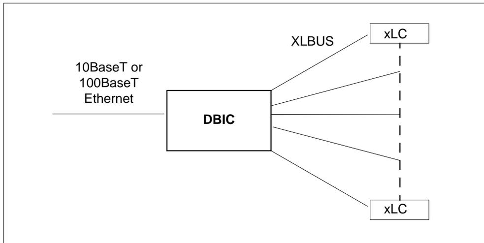
The NTEX54CA supports a transmission rate of 1280 kbit/s downstream and 320 kbit/s upstream. The NTEX54CA supports 10Base T or 100BaseT Ethernet interfaces.
