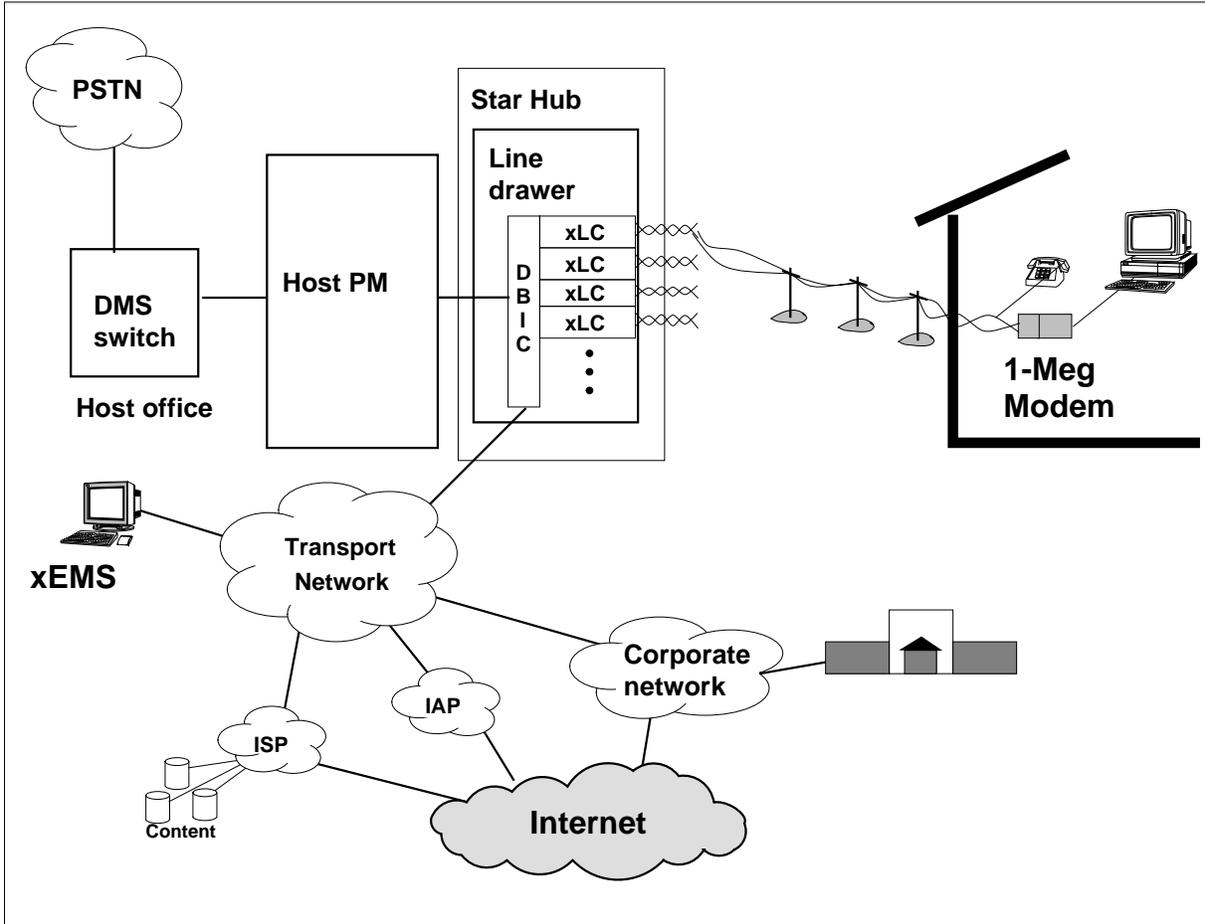
The Star Hub line drawer contains the DBIC and xLCs. The Star Hub can hold up to 18 line drawers. Each line drawer can hold one DBIC and up to 31 xLCs. Each 1-Meg Modem Service subscriber has an xLC. Each line drawer with xLCs must have a DBIC to provide data service. Each DBIC provides an Ethernet connection to the transport network for all subscribers in the line drawer.
