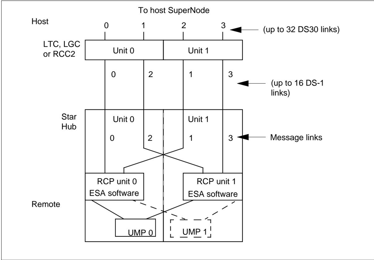
When the Star Hub is in ESA mode, the diagram in this figure is not accurate. In ESA mode, the ESA software that is in the RCP acts as the host peripheral module (PM). In this mode, the host PM is the LTC. This figure does not describe the hardware configuration from the view of the MAP terminal. The Star Hub functions separately from the host.
