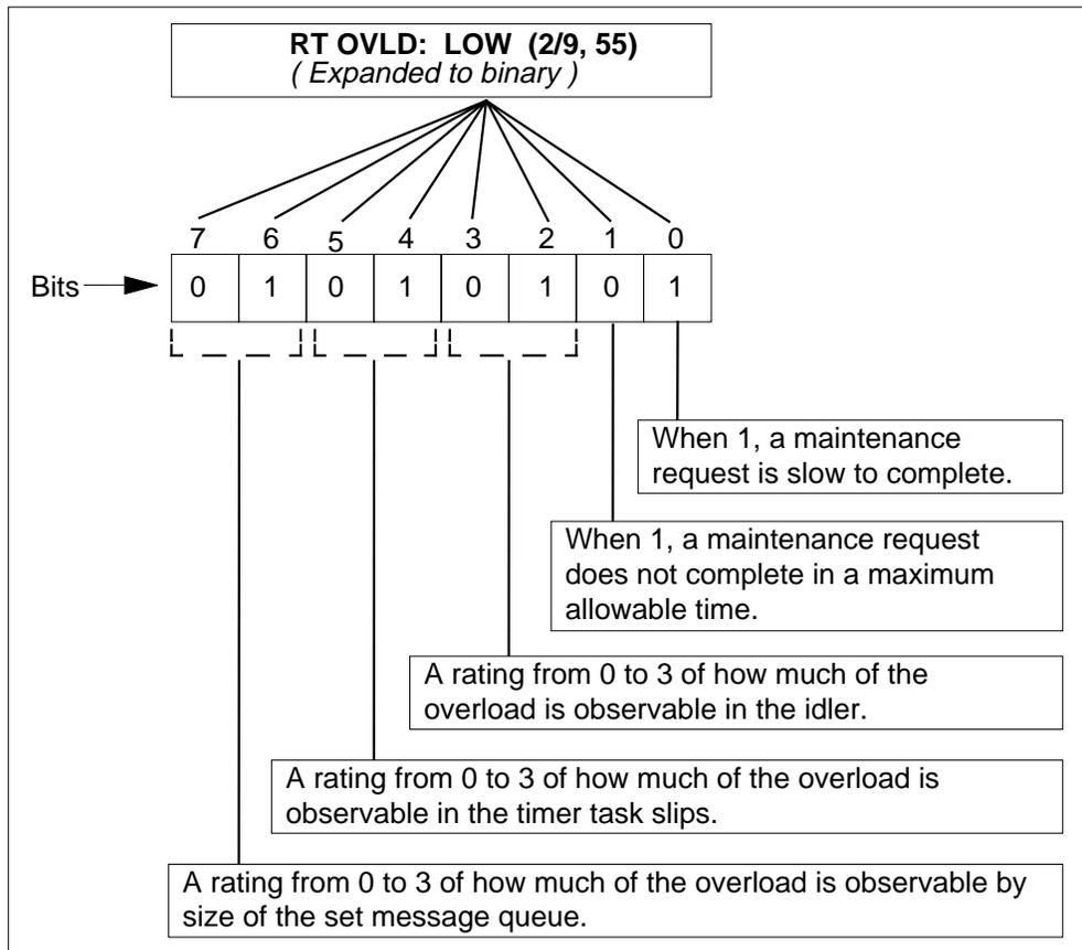
The XLCM maintains overload data that allows the XLCM to provide a summary of the overload period. The XLCM adds this summary to the current overload exit message to the CM. When the CM is at CCM04 or later, this information appears in a modified PM180 LCM Out Of Overload log.
