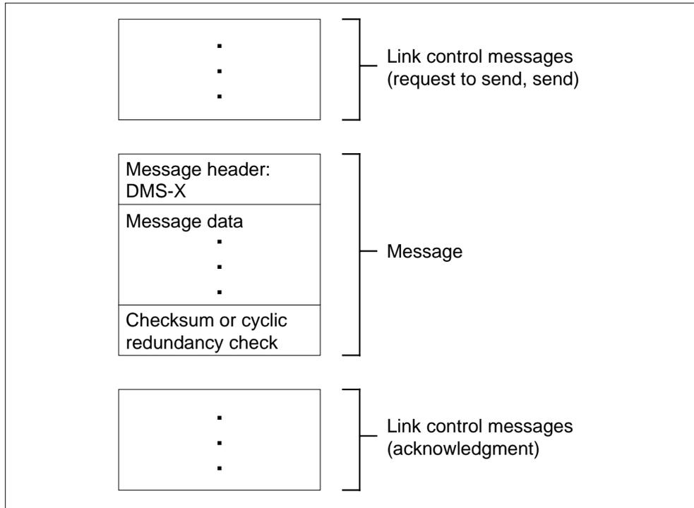
Message time-out and message checksum or CRC calculation perform message error detection. Protocol, checksum or CRC failure can occur on an outgoing message. When this event occurs, the node that attempted the send sequence attempts the send sequence again. On an incoming message failure, the node that sends routes the message again over an alternate (C-side) link. Hardware redundancies provide a minimum of one alternative path to and from a node.
