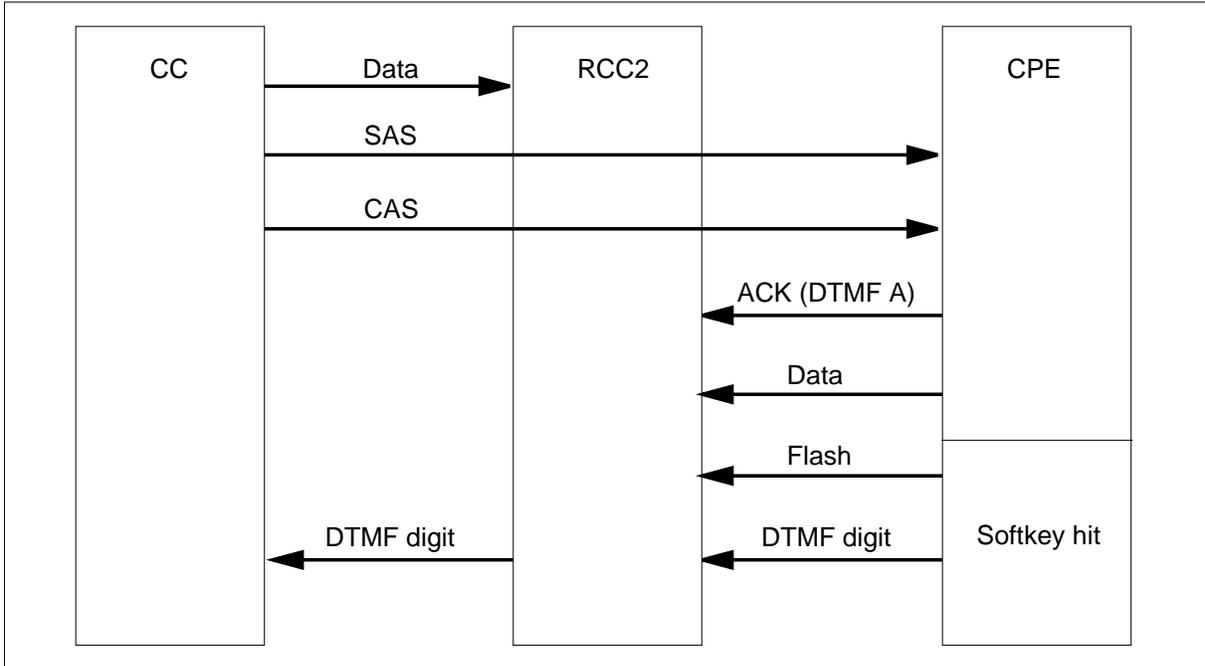
Figure 1-2 Example of a DSCWID call on a SCWID set
