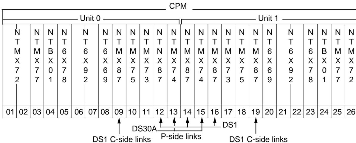
In NA010 and lower, up to 16 C-side ports are available. This configuration requires the NTMX87AA/AB in slots 9 and 19. NA011 and higher supports these packs when an office needs only up to 16 C-side links.
