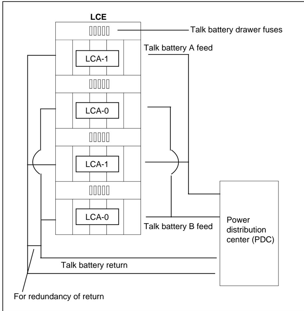
The A feed provides talk battery for the second and fourth shelves of the LCE frame. The B feed provides talk battery for the first and third shelves. The feeds are not redundant. A single fault that loses a feed can affect two shelves. The two shelves can hold a maximum of 640 subscriber lines.
