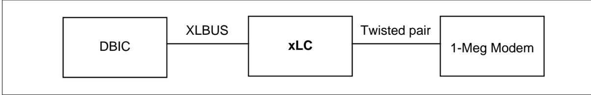
The 1-Meg Modem Service supports three types of xLCs. Each xLC supports different transmission rates and LCM drawer fill requirements. The following table lists the xLCs supported by the 1-Meg Modem Service.
