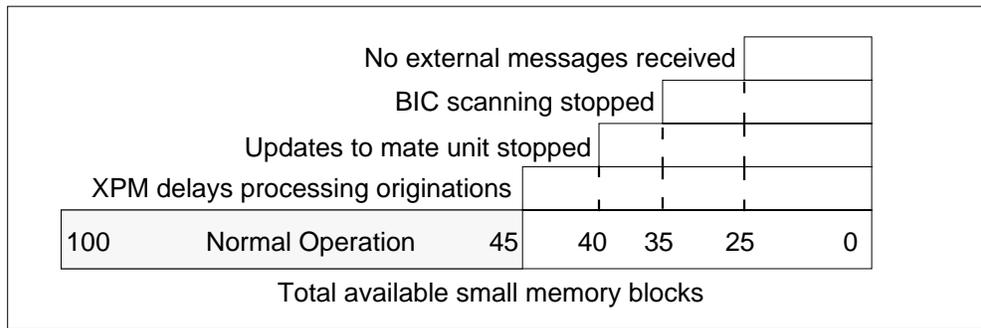
Early models of plain ordinary telephone service (POTS), of the small memory LCM (64 kbyte), show the capacity is memory block limited. In this model, the LCM runs out of small memory blocks before the LCM runs out of real-time use. The design of the LCM depends on this memory block limited capacity. Memory block limited is an LCM characteristic carried over to XLCMs.
