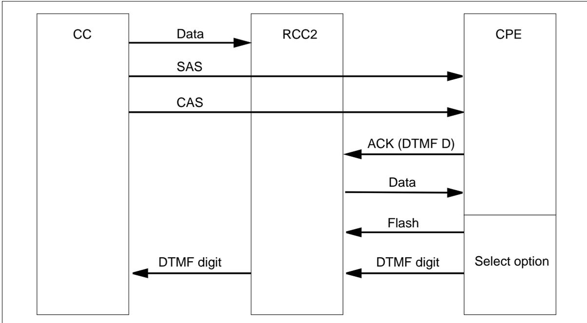
Figure 1-3 Example of a DSCWID call on a 2500 set
