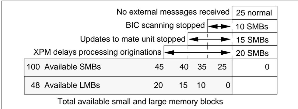
**Changes to the real-time subsystem** The real-time subsystem changes memory block system parameters to keep memory block limits ahead of real-time limits.
