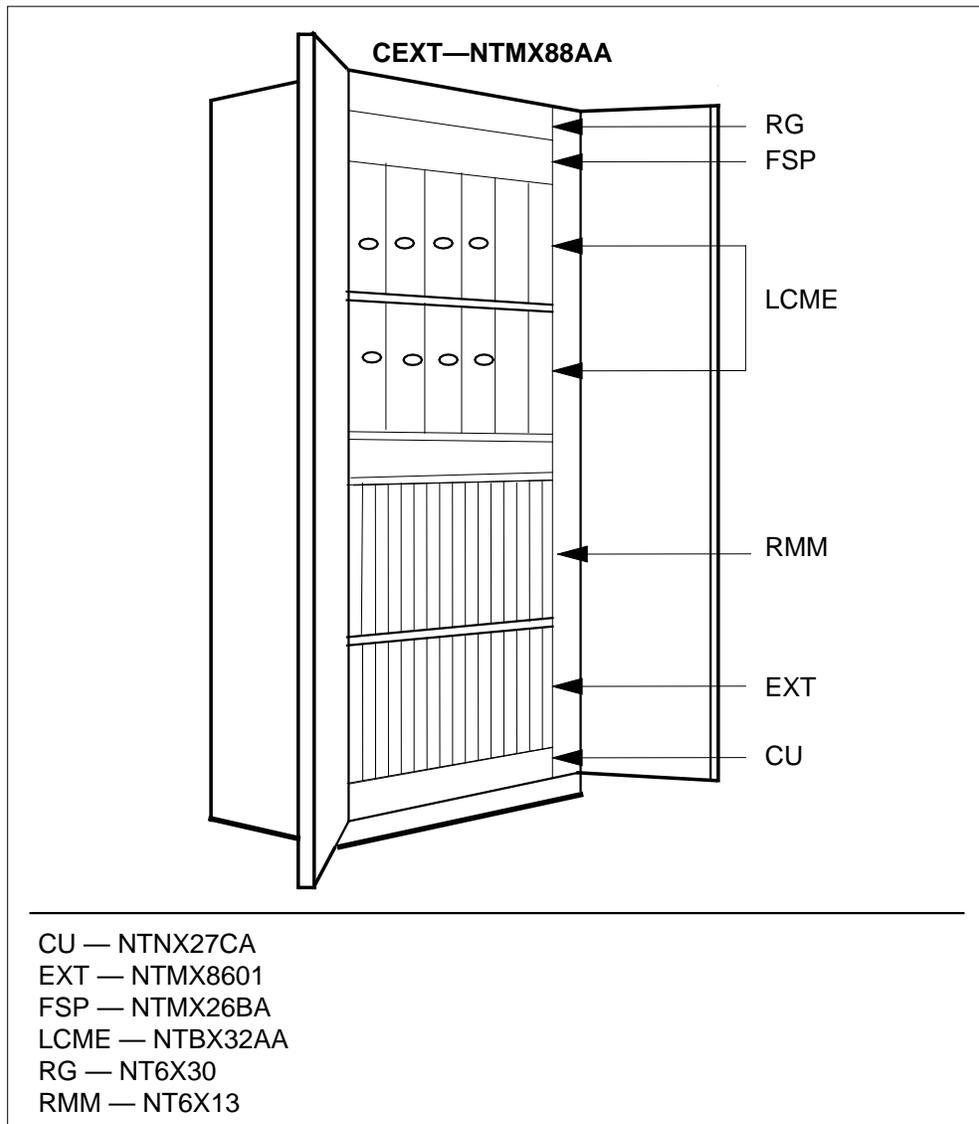
The CEXT provides room for additional DS-1 interfaces and DCH cards. The CEXT units 1 and 2 require the DS60 card that provides DS60 links to the CRSC. The extension card contains 12 DS60 links that connect the card to the RCC2 shelf. The EXT shelf uses two-extension cards.
