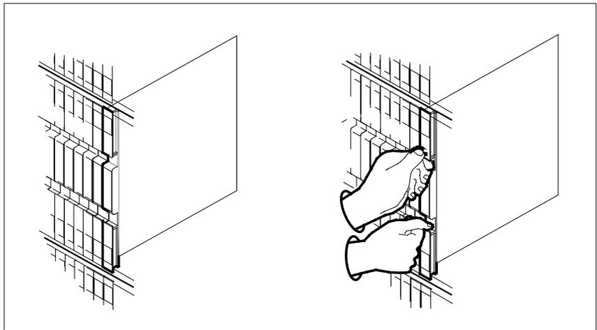
**b** Open the locking levers on the card to be replaced. Carefully pull the card toward you until it clears the shelf.
