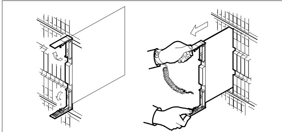
**c** Ensure the replacement card has the same PEC, including suffix, as the card you just removed.
