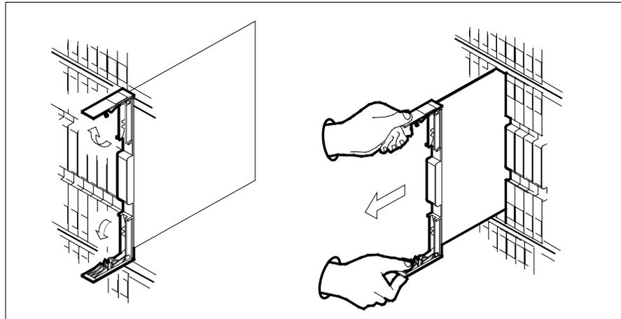
**c** Ensure the replacement card has the same PEC, including suffix, as the card you just removed.
