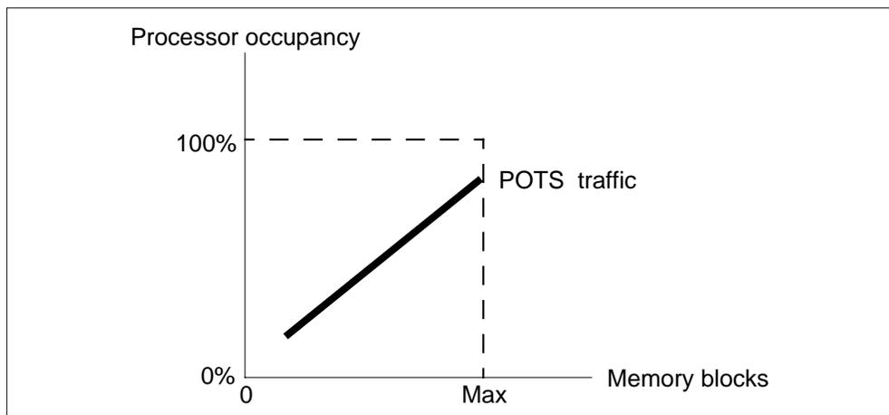
The XLCMs have more memory blocks than small-memory LCMs. The XLCMs must accommodate additional messaging requirements. An example of additional requirements are P-phones provisioned with features like
