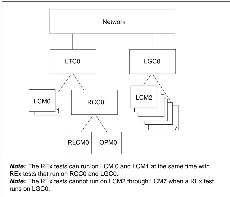
The separation of the LCM\_REX\_TEST and the LCMCOV\_REX\_TEST allows faster completion of site REX\_TEST cover. The LCM\_REX\_TESTS can run without the limits of the converter voltage and ring tests. The LCM\_REX\_TESTS can run at the same time and scheduled separately for the best execution periods.
