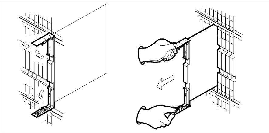
**c** Ensure the replacement card has the same PEC, including suffix, as the card you just removed.
