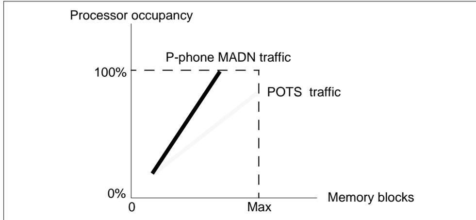
**Figure 1-19 Processor occupancy—memory block reduction after real-time overload detection**
