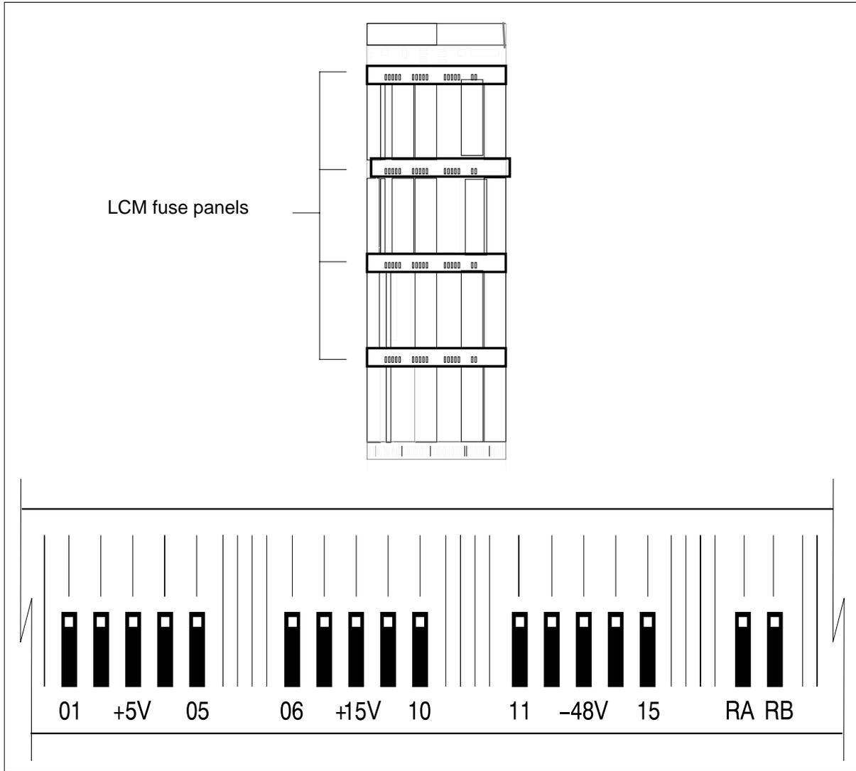
**Note:** Fuses are coded for position. The colored square on the face of the fuse identifies the top edge.
