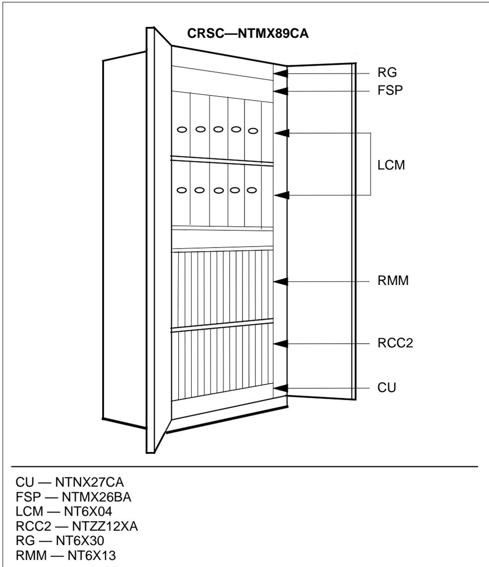
**Enhanced remote cluster controller 2** The RSC-S is based on the RCC2. The RCC2 is the master controller for RSC-S peripherals. The RCC2 controls associated LCMs, RMMs, remotes, and digital trunks as the host directs.
