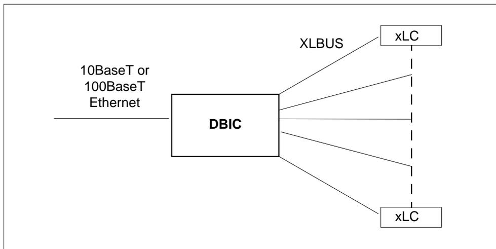
The 1-Meg Modem Service supports three types of DBICs. Each DBIC supports different transmission rates and Ethernet interfaces. The following table lists the DBICs supported by the 1-Meg Modem Service.
