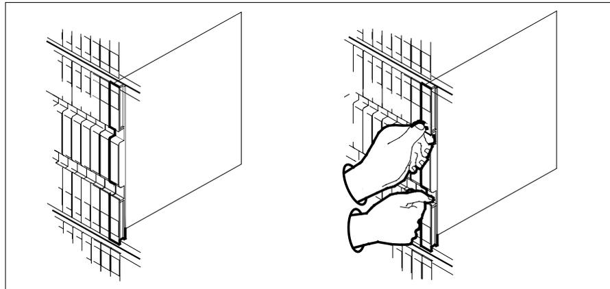
**b** Open the locking levers on the card to be replaced and gently pull the card toward you until it clears the shelf.
