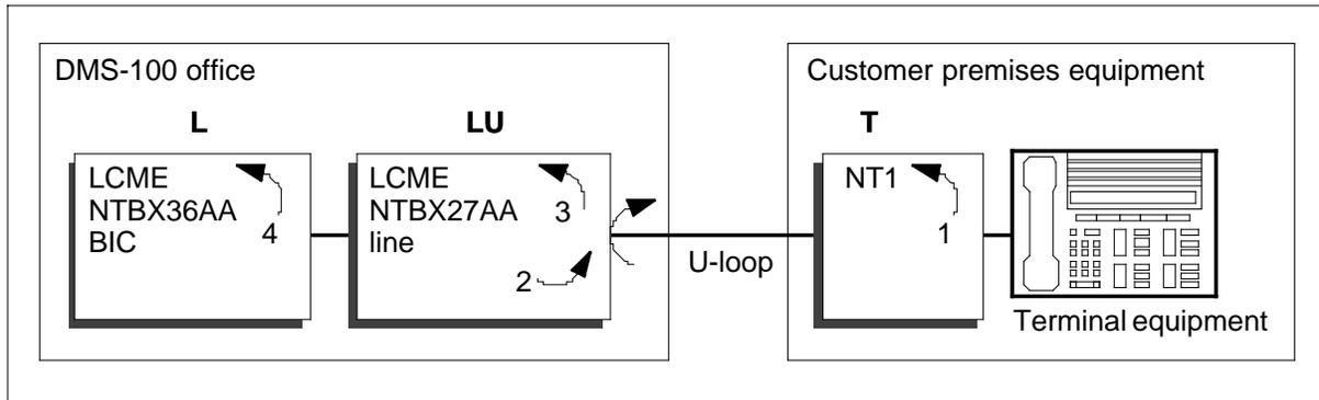
**Note:** A fourth loopback point is available if the 2B1Q lines are equipped with MP-EOC line units. Use a BERT to verify the low-level operation of the line to the CPE. The M5317T and M5209T sets can operate the loopback functions without any of the service profile identifiers (SPID), terminal endpoint identifiers (TEI), or DNs programmed on the set.
