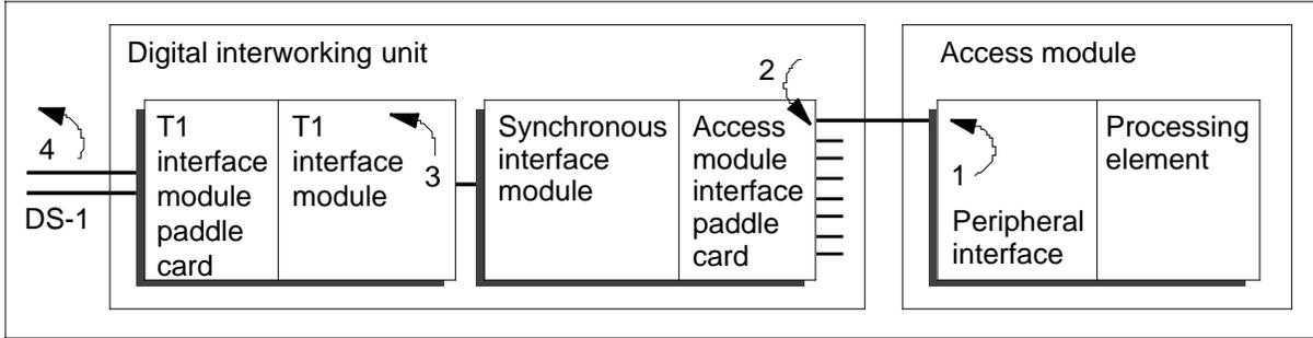
Set all the software-controlled loopback points using the operator commands at the network control system (NCS) operator console or at the AM local operator console.
