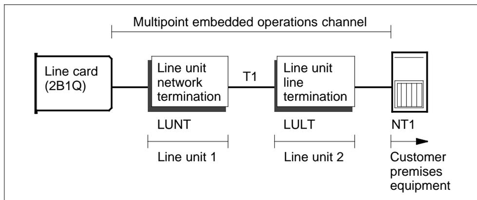
A line unit line termination (LULT) is connected on the NT1 side. The LULT transfers unaltered EOC signals from the T1 to the ISDN line. Up to eight line units or four sets (LUNT and LULT) can be provided on an ISDN 2B1Q loop. You can display the number of line units on a MP-EOC LEN by entering the QLEN command.
