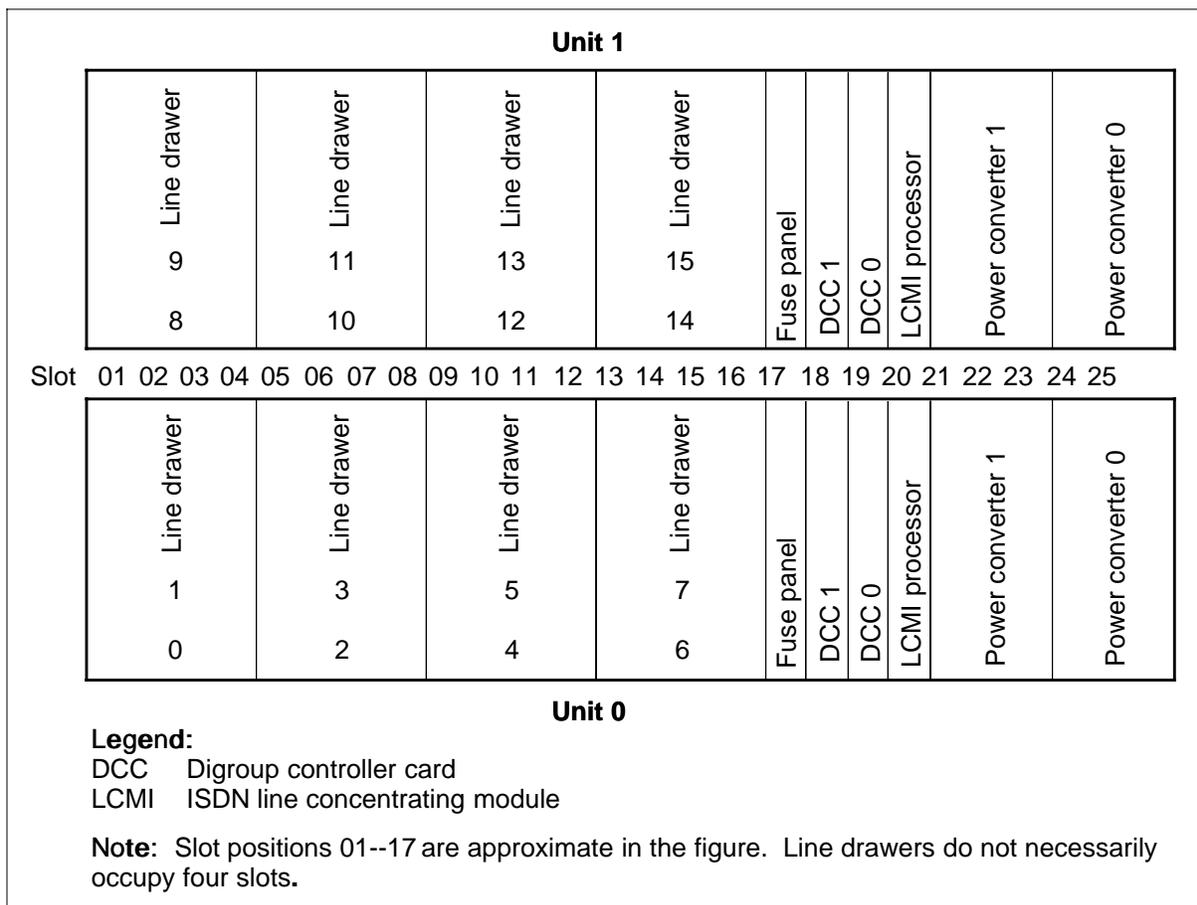
Figure 7-2 Physical and logical layout of the LCME line drawer
