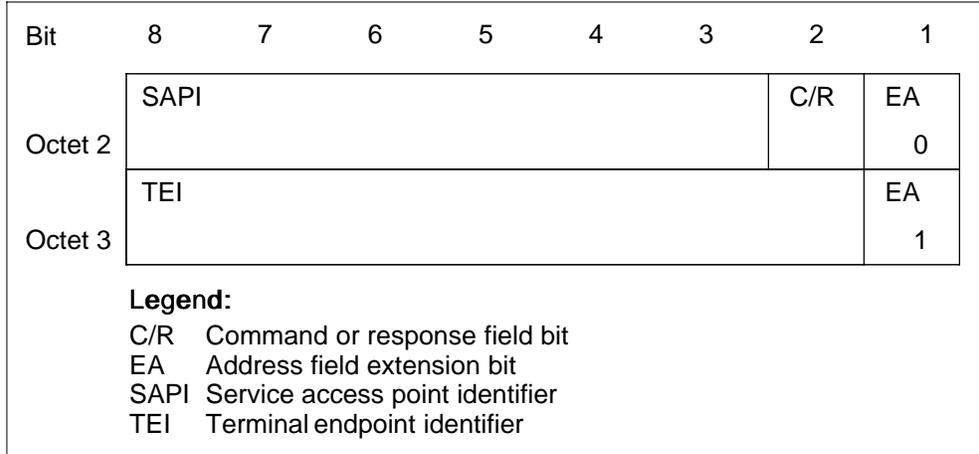
The SAPI identifies the type of message that is being sent. The C/R bit identifies the frame as either a command or a response. The TEI identifies the logical ISDN terminal. Table 8-1, 8-2, and 8-3 list the possible values for each of these items.
