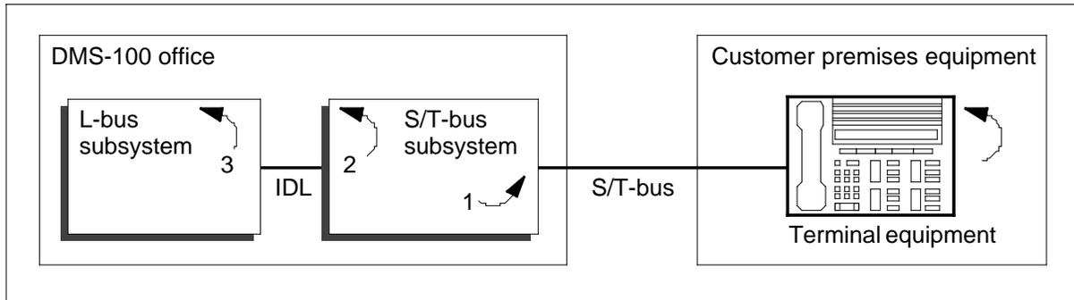
**Note:** Use a BERT to verify the low-level operation of the line to the CPE. The M5317T and M5209T sets can operate the loopback functions without any of the SPIDs, TEIs, or directory numbers programmed on the set.
