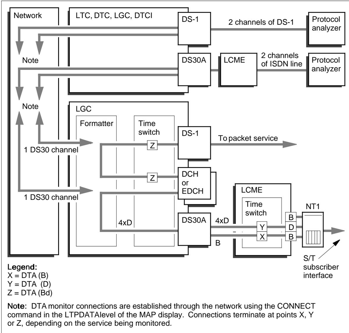
Each loop is allowed only one DTA Bd connection at a time. However, there can be multiple taps on one Bd connection so that different loops using the same Bd connection have DTA Bd connections.
