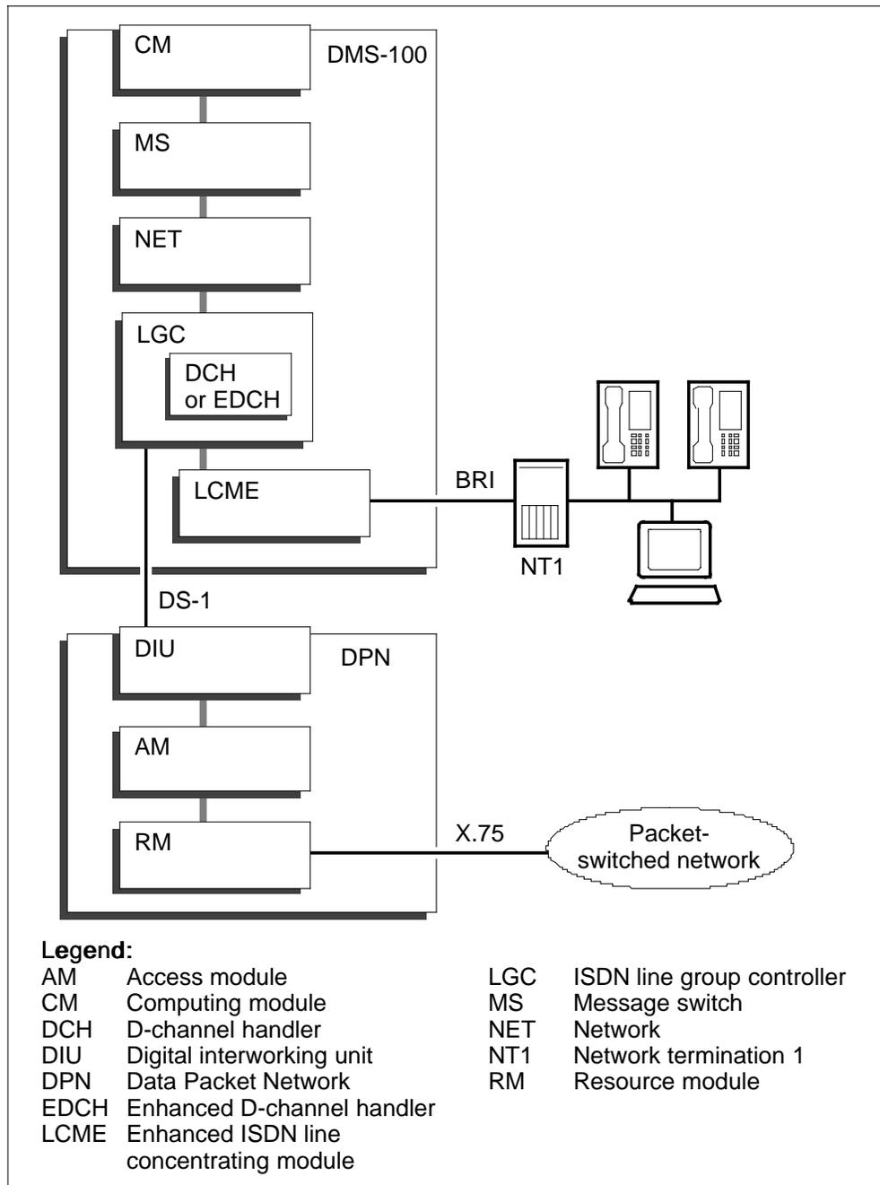
Figure 1-2 Key components of a DMS-100 ISDN using a DMS packet handler
